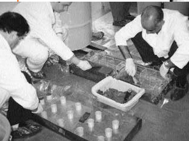
**Preparation of specimens for leach and compression tests.**
