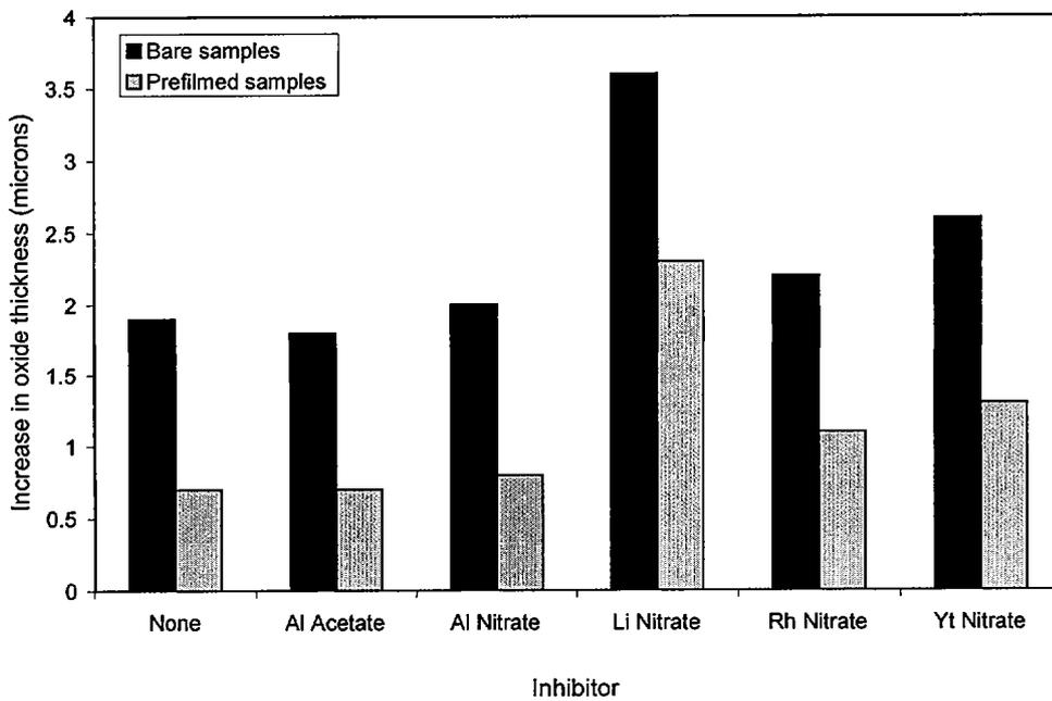
Figure 2 Increase in oxide thickness for both bare and prefilled samples for various inhibiting additions compared with the reference solution (none).
