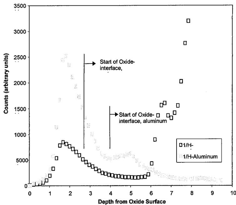
Figure 4 Through-oxide-thickness depth profile by SIMS of mass 1 (H) showing significant reduction in H uptake by the bulk alloy for a bare sample exposed to a nitrate-containing solution compared to the reference solution.
