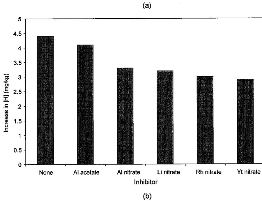
Figure 1 Increase in [H] for various inhibiting additions compared with the reference solution (none) for (a) bare and (b) prefilled samples.
