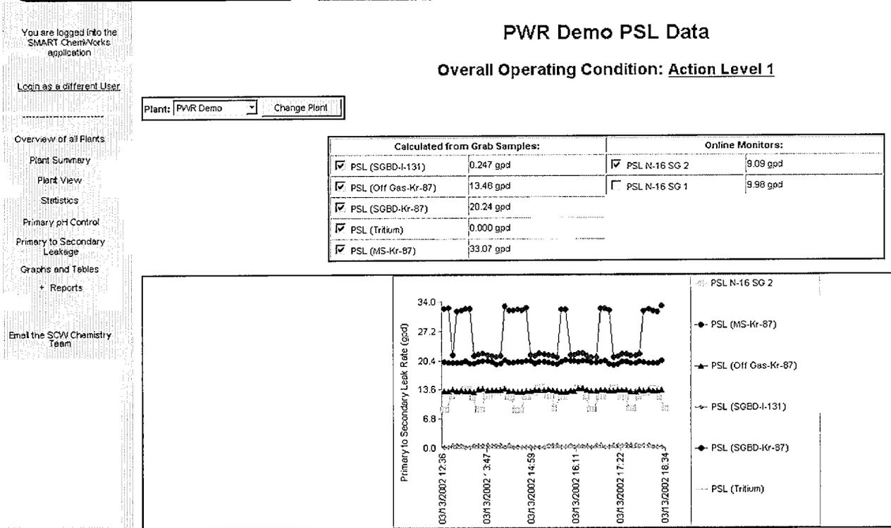
**Figure 3 Primary to Secondary Leakage Monitoring**
