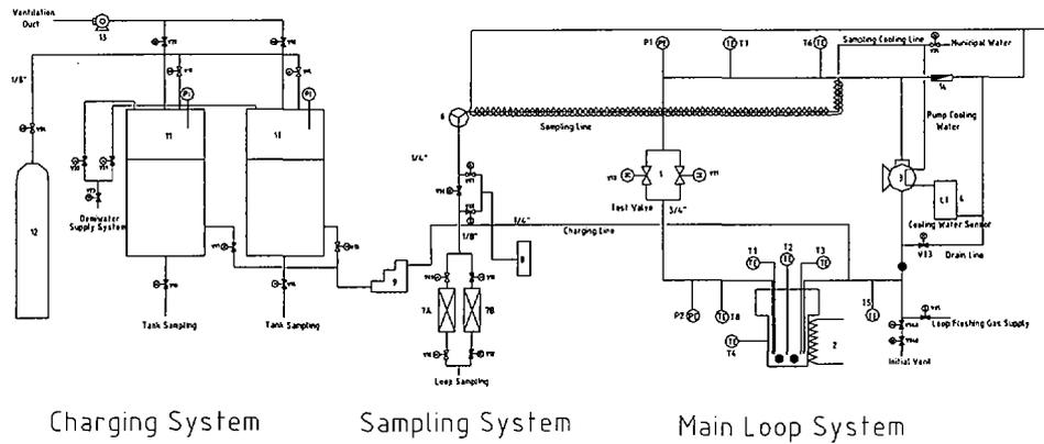
Figure 2. Schematic diagram of HT/HP valve test loop.
