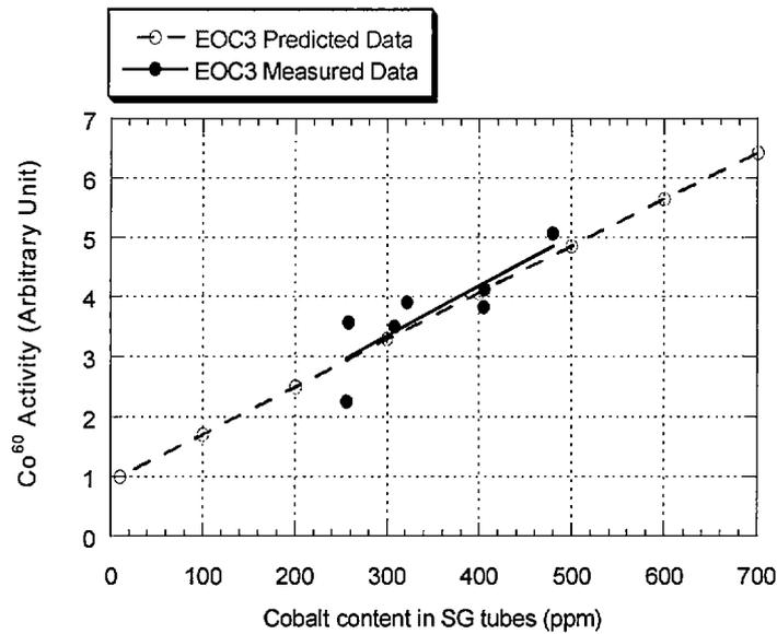
Figure 11. CREAT prediction results in comparison of the French plant data for the surface activity as a function of Co content in SG tubings.
