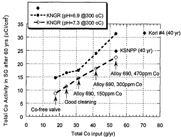
Figure 17. Surface activity at the end of plant life as a function of total Co input.
