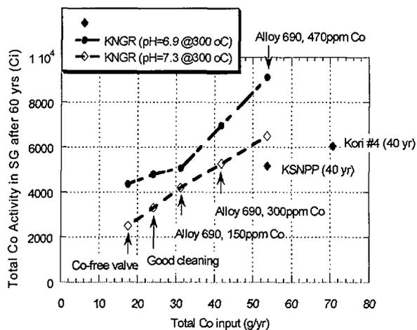
Figure 18. Overall activity at the end of plant life as a function of total Co input.
