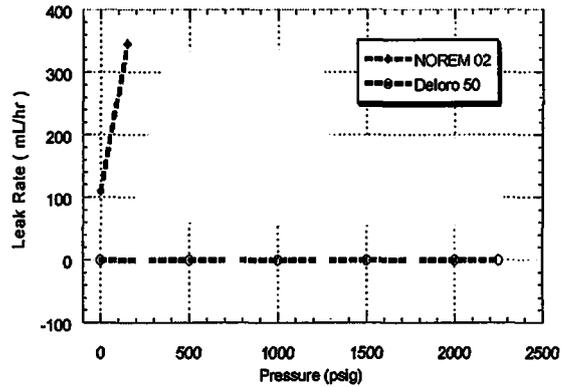
Figure 5. Cold leak test results posterior to 1,000 cycles test as a function of pressure.
