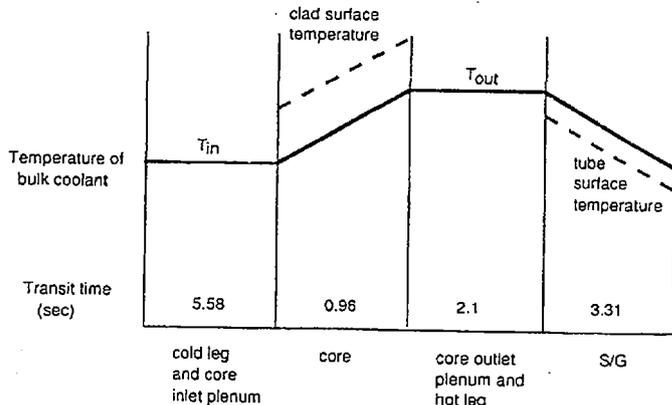
Figure 9. Temperature distribution of primary coolant as a function of location [9].
