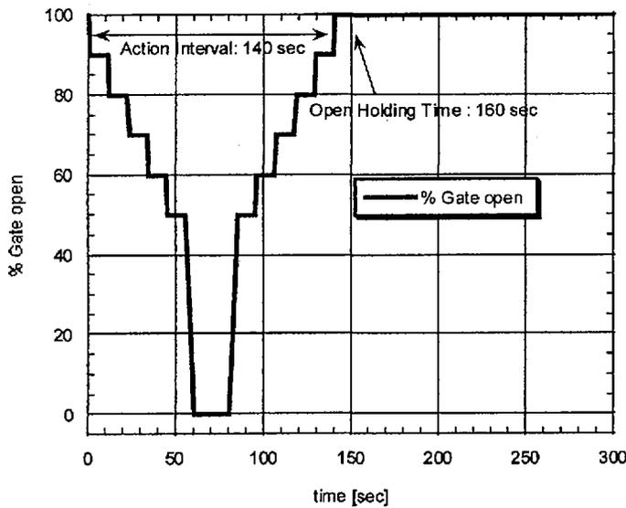
Figure 3. Fraction of gate opening as a function of time during one cycle.
