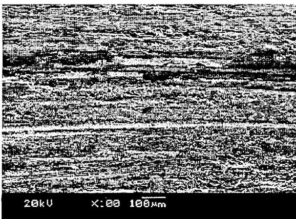
Figure 7. SEM micrograph of the worn surface of NOREM 02 disc after 1,000 cycles test.
