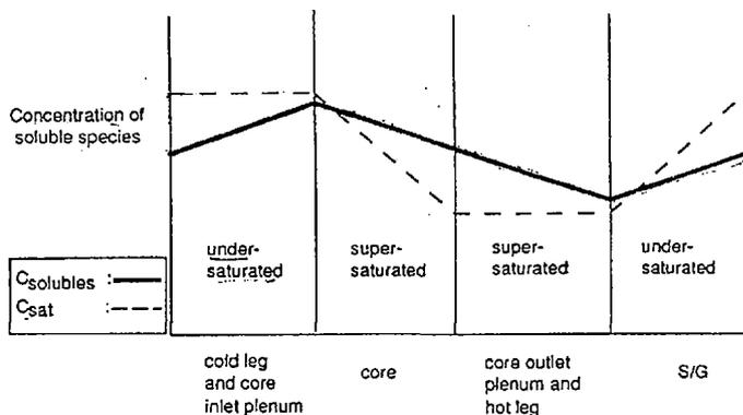
Figure 10. Concentration of soluble crud in primary coolant as a function of location [9].
