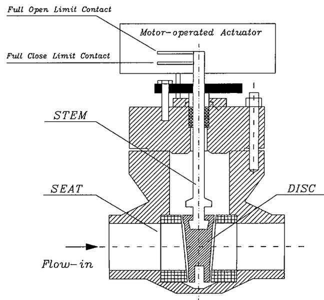
Figure 1. Cross sectional view of the 3/4" test gate valve.
