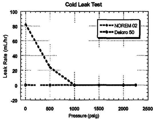
Figure 4. Cold leak test results prior to cycling test as a function of pressure.
