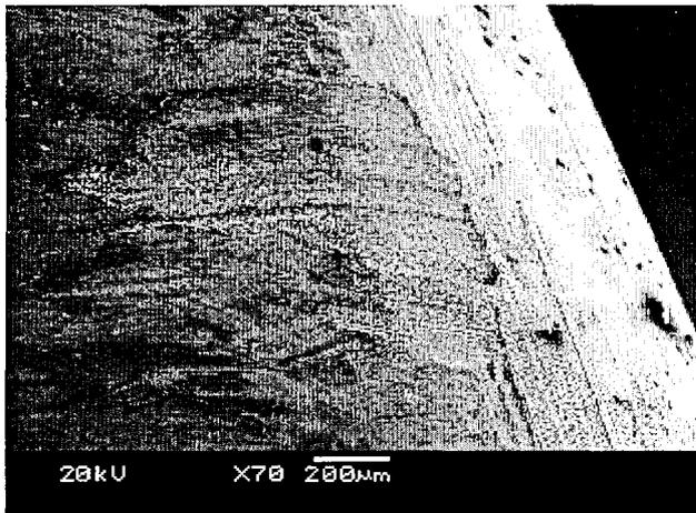
Figure 6. SEM micrograph of the edge of NOREM 02 disc after 1,000 cycles test.
