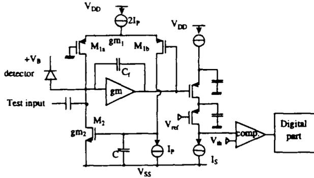
Fig. 4: Schematic of the analogue front-end of a pixel detector.
