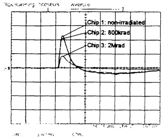
Fig. 6: Pulse response measured at shaper output (5mV/div, 100ns/div)
