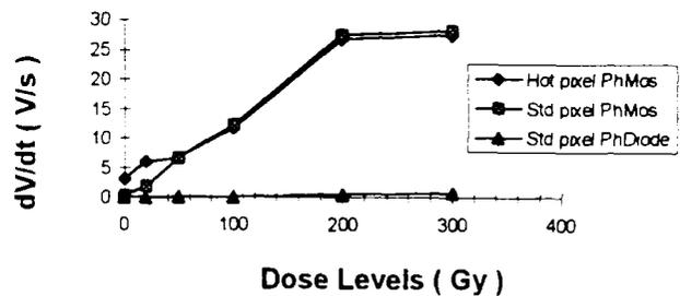
Figure 4: Dose Level Effects on Dark Current for the PhotoMos and the Photodiode.
