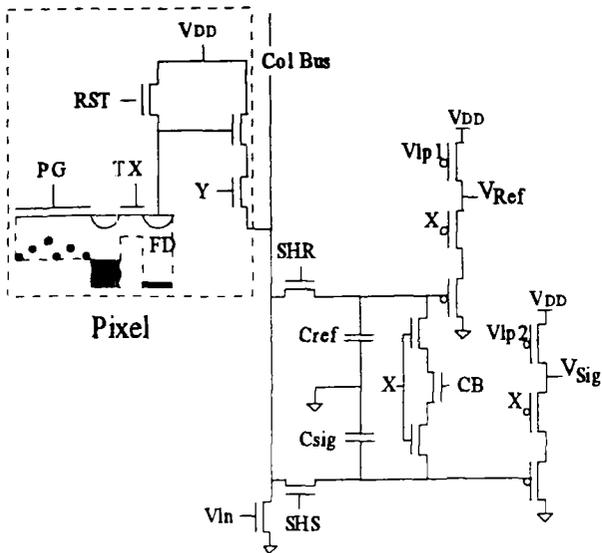
Figure 2 : APS photoMos pixel and readout circuit.
