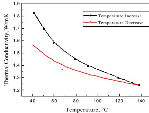
Fig 3: Thermal conductivity of concrete B-300 versus average temperature
