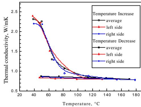
Fig 2: Thermal conductivity of mortar versus average temperature
