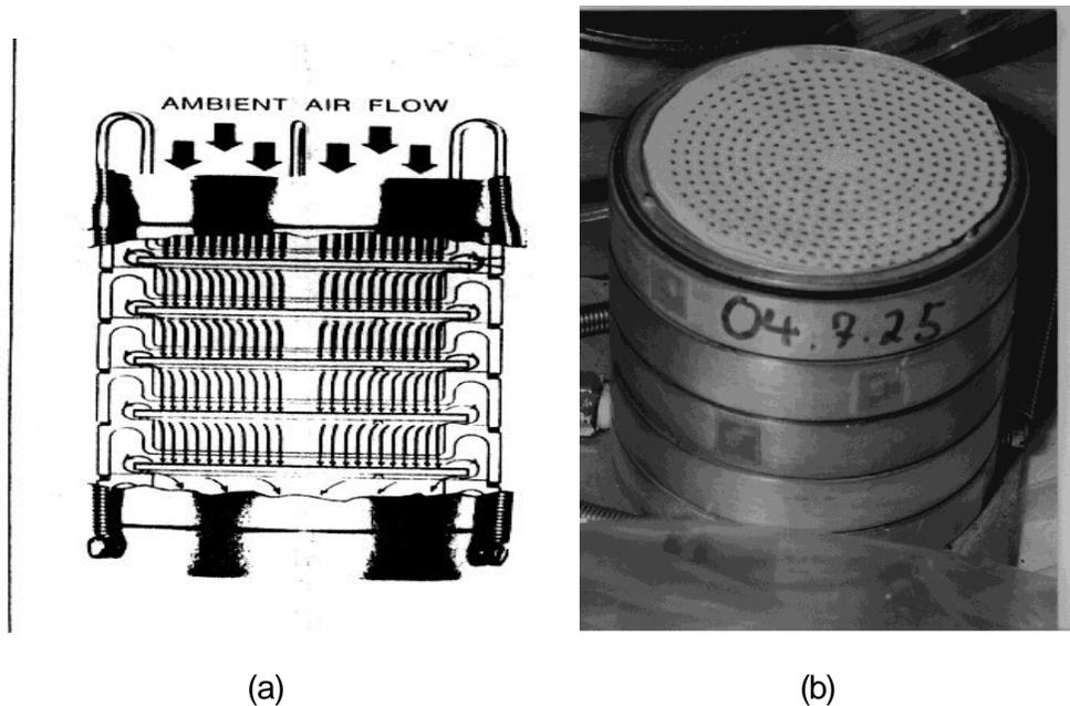
Fig. 1. (a) Schematic description and (b) a picture of the cascade impactor.
