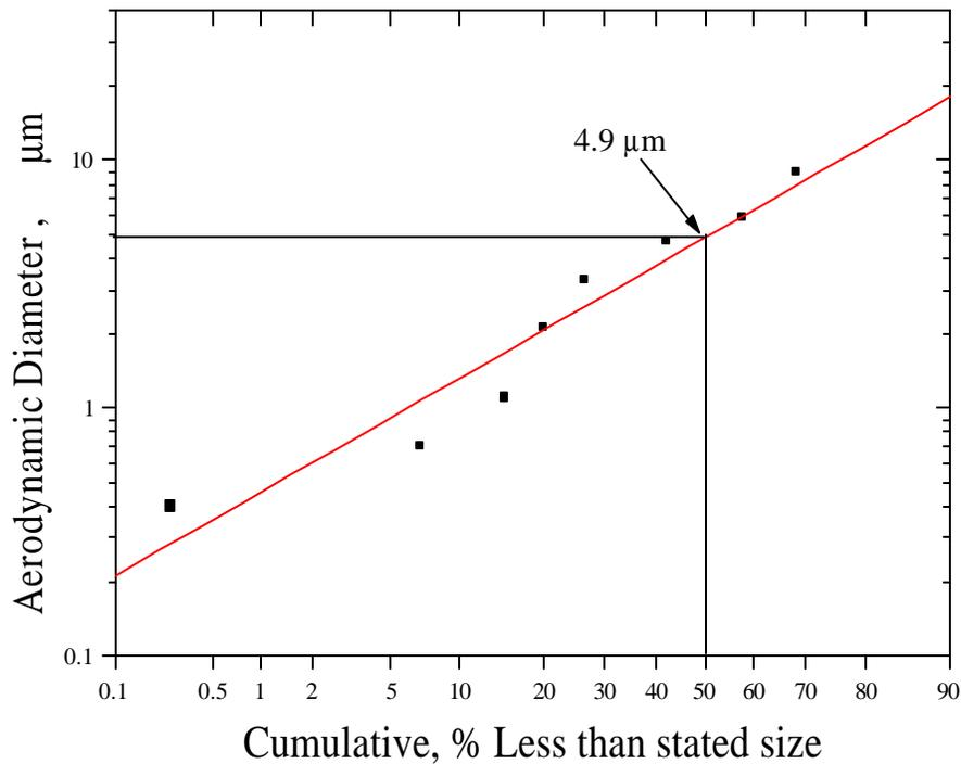
Fig. 2. The distribution of radioactive aerosol's aerodynamic diameter as measured near the conversion process of  $UO_3$  into  $UF_4$  powder.
