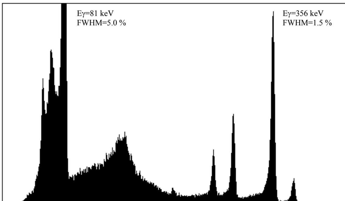
**Figure 1.** Combined spectrum of corrected pad signals for  $1\text{cm} \times 1\text{cm} \times 1\text{cm}$  Pixellated CdZnTe Gamma Detector illuminated with a  $^{133}\text{Ba}$  source.
