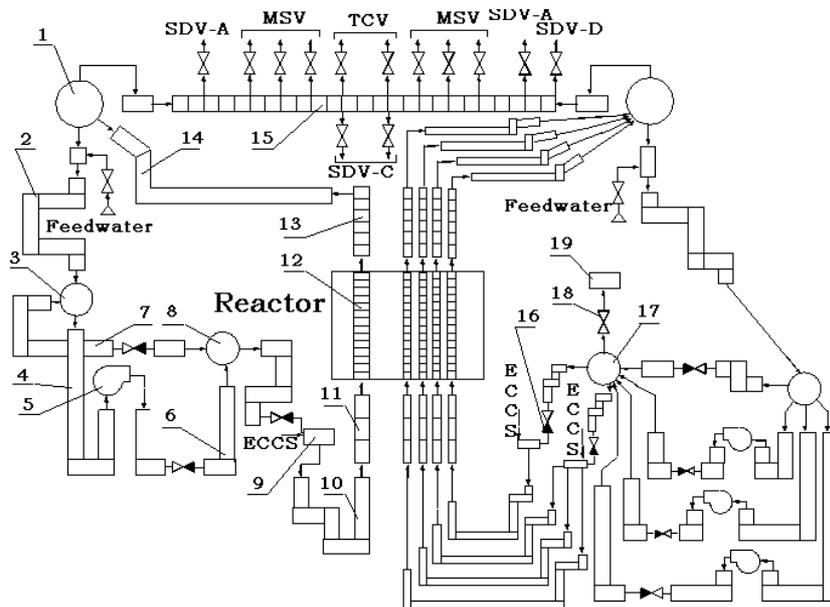
**Figure 1 RELAP5 Ignalina NPP model nodalization scheme:**
