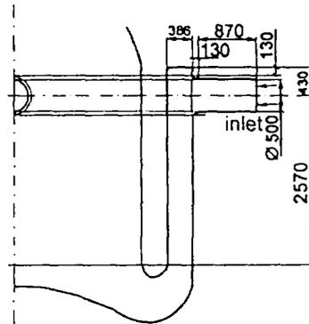
Figure 4. Geometry of the downcomer and the horizontal inlet nozzles
