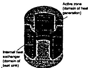
Figure 16. Model of a reactor with internal heat exchangers
