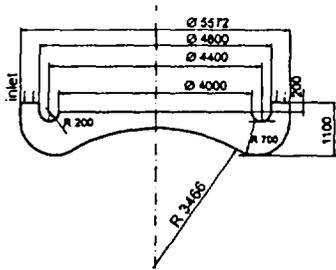
Figure 2. Geometry of the lower plenum
