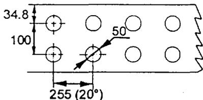
Figure 32. Geometry of the perforated wall model
