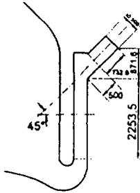
Figure 10. Geometry with 45-degree-inlet
