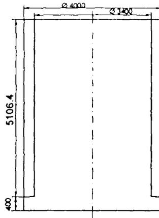
Figure 25. Dimensions of a reactor with a one-volume internal heat exchanger on the perimeter
