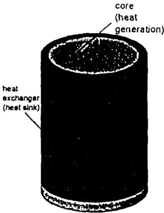
Figure 24. Model of a reactor with a one-volume internal heat exchanger on the perimeter
