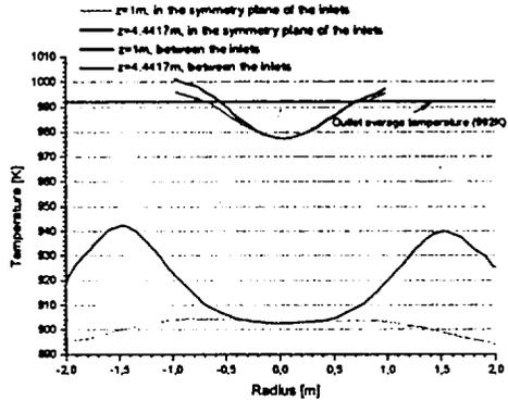
Figure 9. Radial distributions of the temperature in the core (horizontal inlet)
