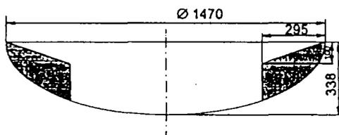
Figure 30. Geometry of the lower plenum
