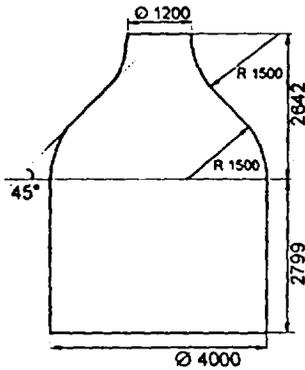
Figure 1. Geometry of the core
