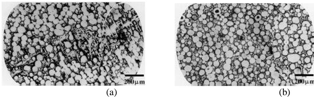
Figure 9. Microstructures of extruded fuel meats containing 50 volume % atomized  $U_3Si$  powder mixed by (a) off-axis rotating drum mixer showing inhomogeneous distribution of  $U_3Si$  and (b) V-shape tumbling mixer showing homogeneous distribution of  $U_3Si$  particles.
