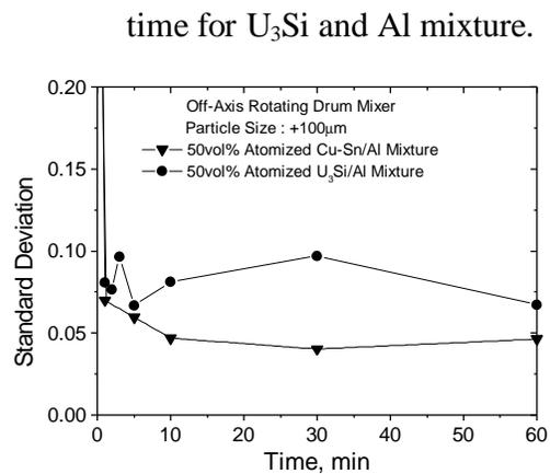
Figure 3. The homogeneities of  $\text{U}_3\text{Si}/\text{Al}$  and Cu-Sn/Al mixture with two kinds
