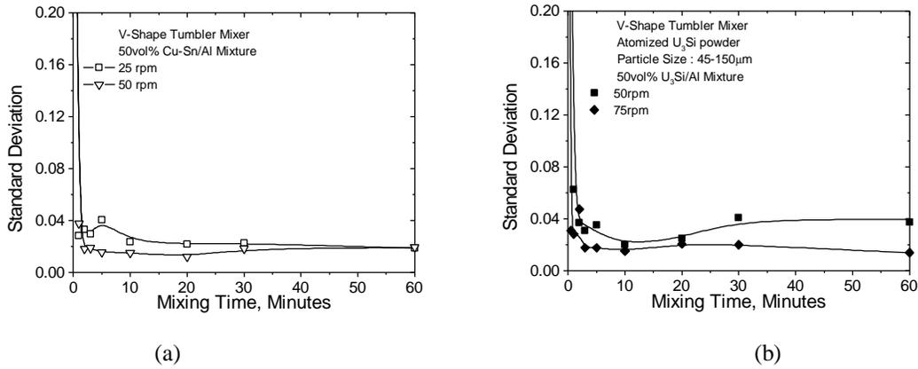
Figure 7. The variation of the standard deviation is compared for two kinds of rotating speeds time. (a) 25 and 50 rpm for Cu-Sn/Al mixture and (b) 50 and 75 rpm for  $U_3Si$ /Al mixture.
