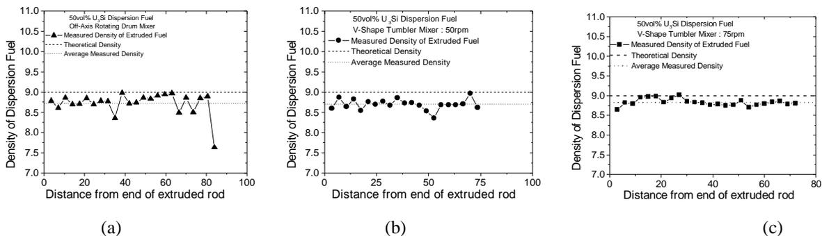
Figure 8. The variation of the density of samples sliced along the extruded fuel rod.
