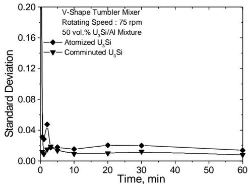
Figure 2. The variation of the standard deviation of the measured apparent densities is shown with
