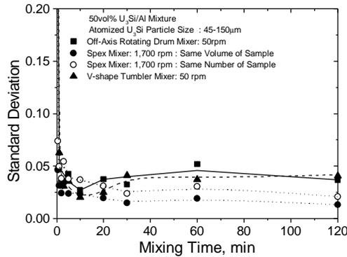
Figure 5. The variation of the standard deviations of the measured apparent densities is shown with time.
