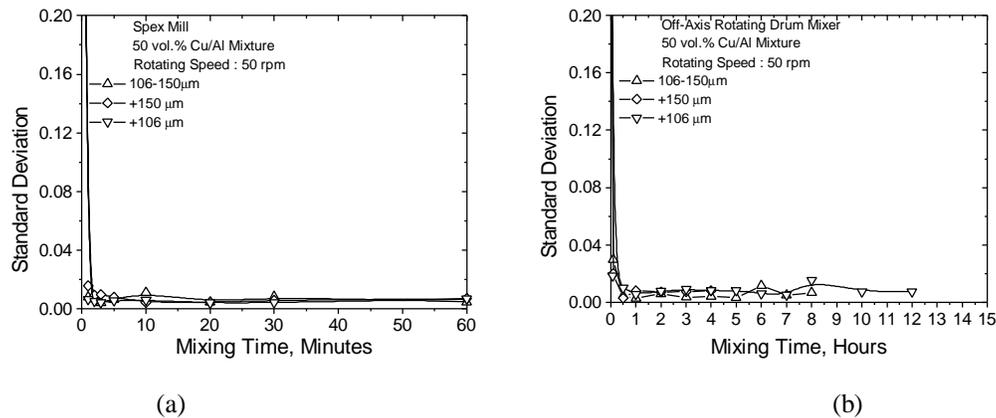
Figure 4. The variation of standard deviation of irregular Cu having different size distributions and Al mixtures are shown with time. (a) Spex mill mixer and (b) off-axis rotating drum mixer.
