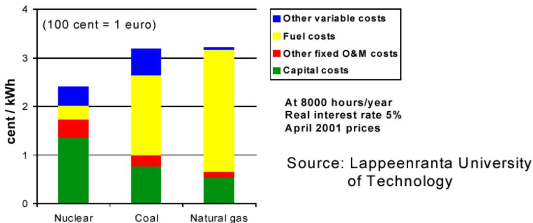
Figure 3 Generating costs of different base-load production alternatives in Finland [17]
