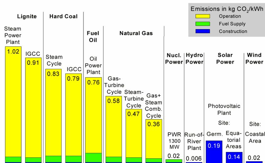
Figure 5 Greenhouse Gas Emissions from Electricity Production per kWh (Source: Siemens/Voss/VDI-GET)
