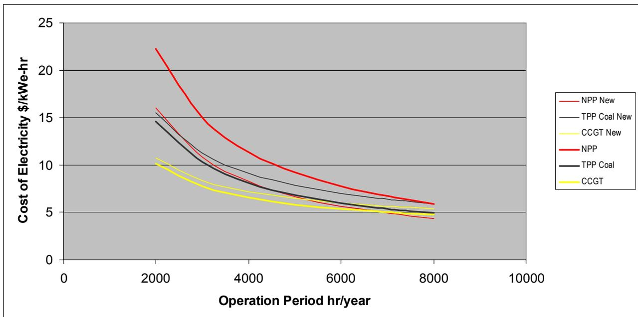
Figure 5 Reduction of NPP Overnight Cost, Construction Period from 5 to 4 years and included carbon taxes
