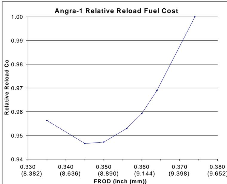
Figure 2. Relative Reload Uranium Cost for 340 EFPD and Reload Batch of 40 FA (Reference 5)
