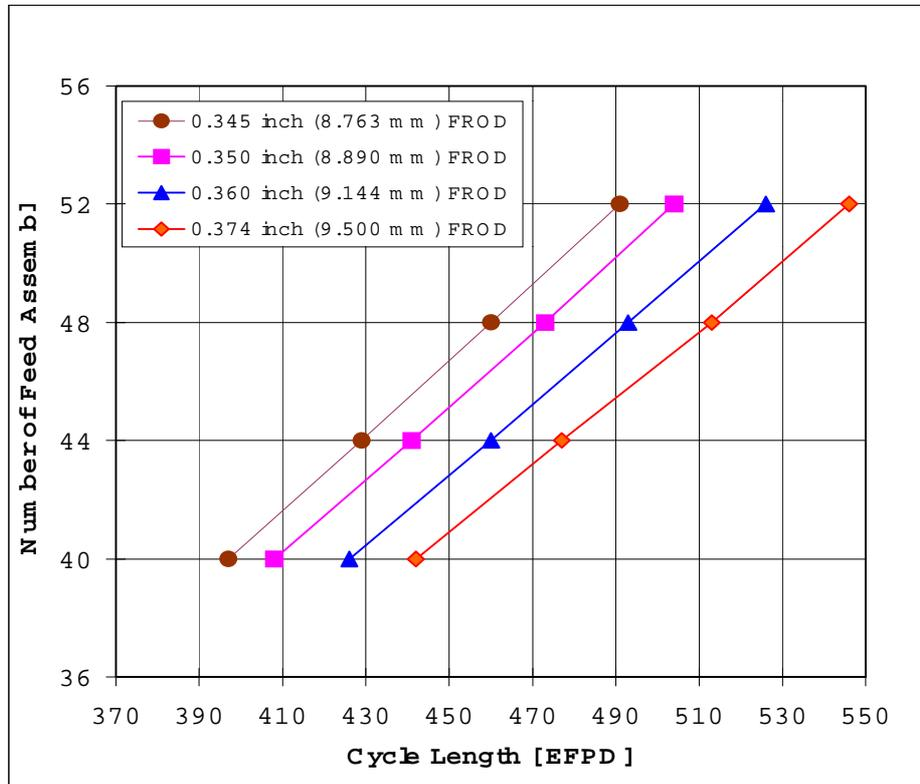
Figure 3. Fuel Cycle Management Approach for Numbers of Feed Assemblies versus EFPD for Reload Batches of 40, 44, 48, and 52 FAs (Reference 5)
