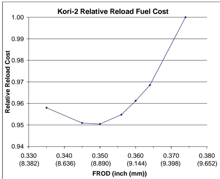
Figure 1. Relative Reload Uranium Cost for 430 EFPD and Reload Batch of 48 FA (Reference 5)
