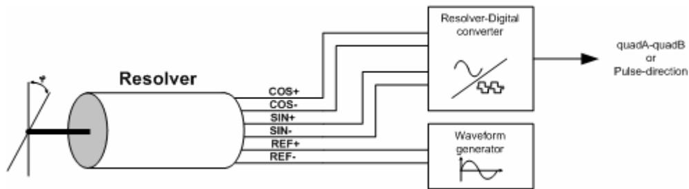
Figure 5. Resolver-to-digital converter
