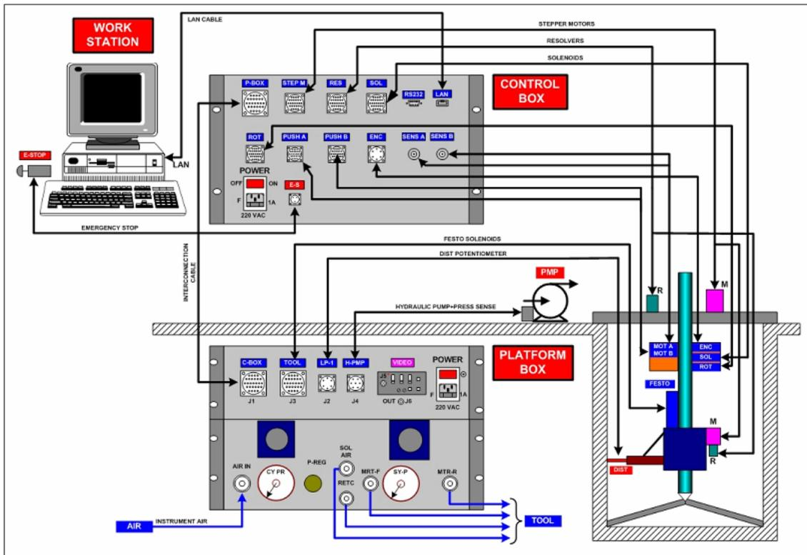
Figure 3. Interconnection schema of the inspection system in a Paks Nuclear power plant
