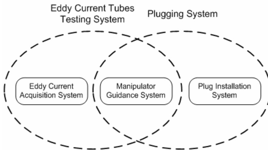
Figure 2. System for the inspection of the VVER steam generator
