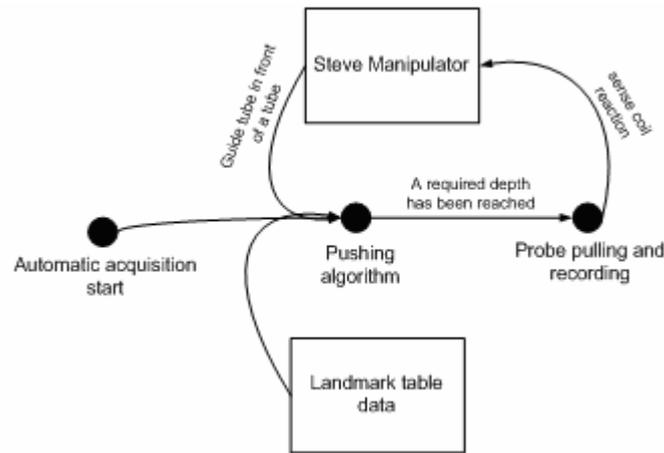
Figure 13. The automatic acquisition process
