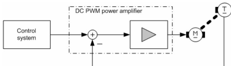
Figure 8. Pusher motors servo loop
