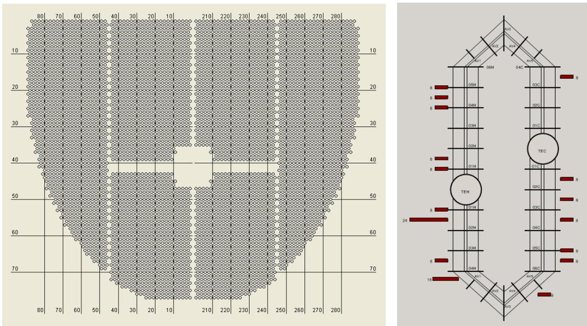
Figure 11. Tube sheet model and top tubes plan
