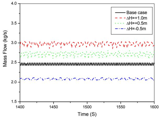
Fig. 6 Steam generator inlet mass flow for the height change.
