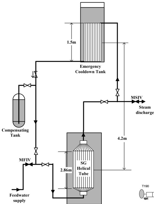
Fig. 1 PRHRS schematic diagram for the SMART
