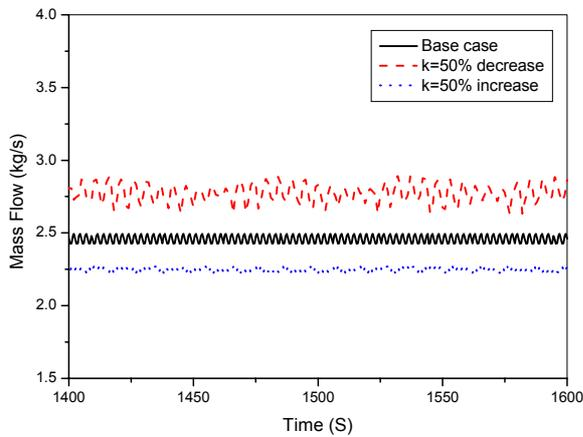
Fig. 7 Steam generator inlet mass flow for the hydraulic resistance change
