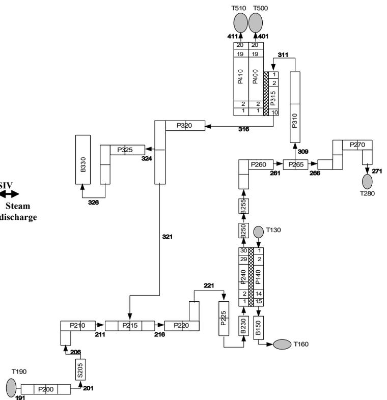
Fig. 2 MARS nodalization for the PRHRS
