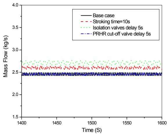
Fig. 8 Steam generator inlet mass flow for the valve actuation time change
