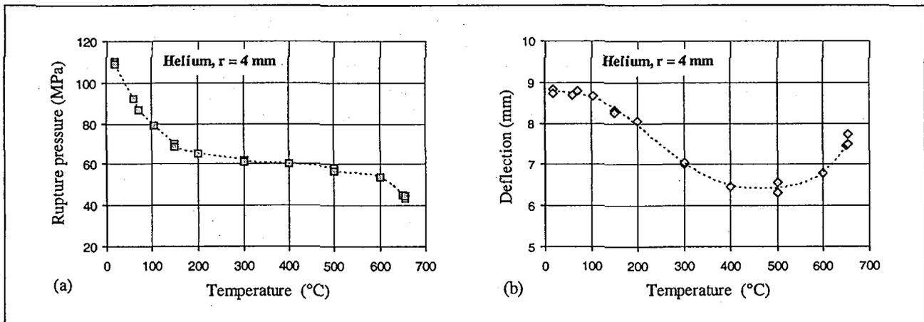
Figure 4: Influence of temperature on the rupture pressure (a) and deflection (b) in biaxial tensile testing.
