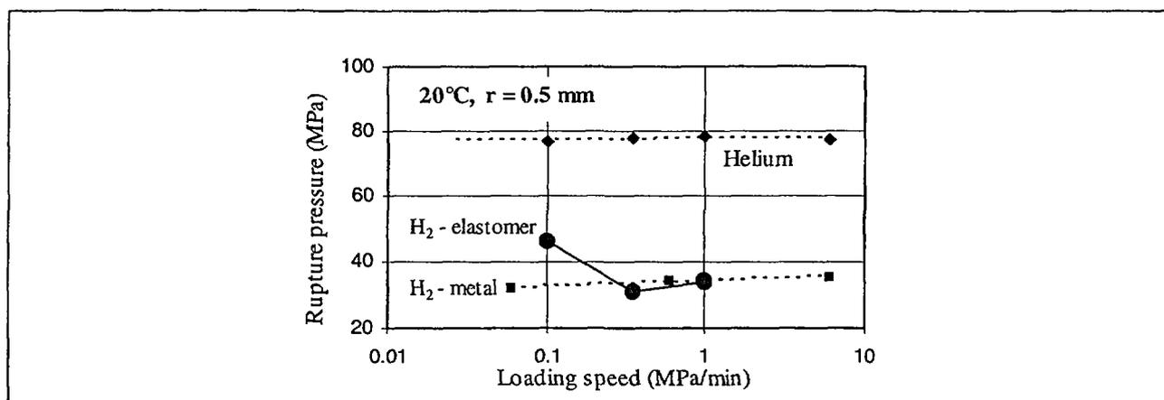
**Figure 3:** Effect of hydrogen purity on the rupture pressures: pure hydrogen in the case of tests realised with a metallic O-ring; polluted hydrogen in the case of test realised with an elastomer O-ring.
