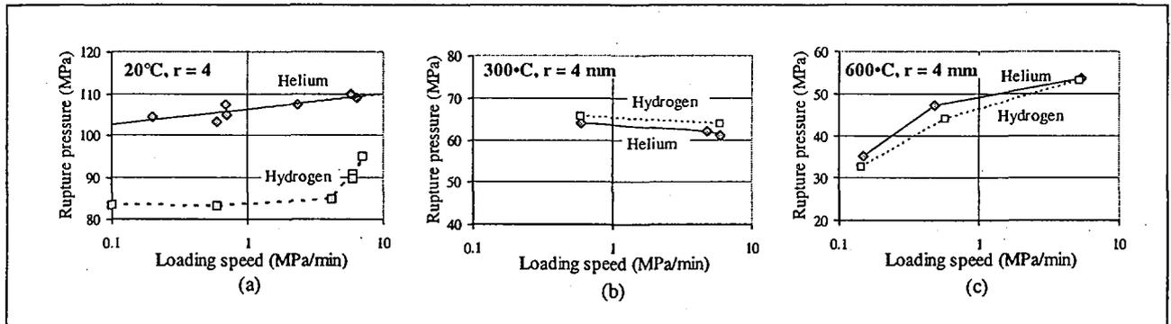
Figure 5: Influence of loading speed and hydrogen on the rupture pressures at three temperature levels: (a) 20°C, (b) 300°C, (c) 600°C.
