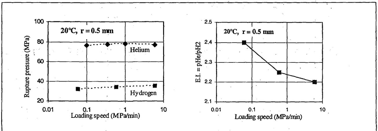
Figure 2: Effect of loading speed on the rupture pressures and embrittlement index E.I.
