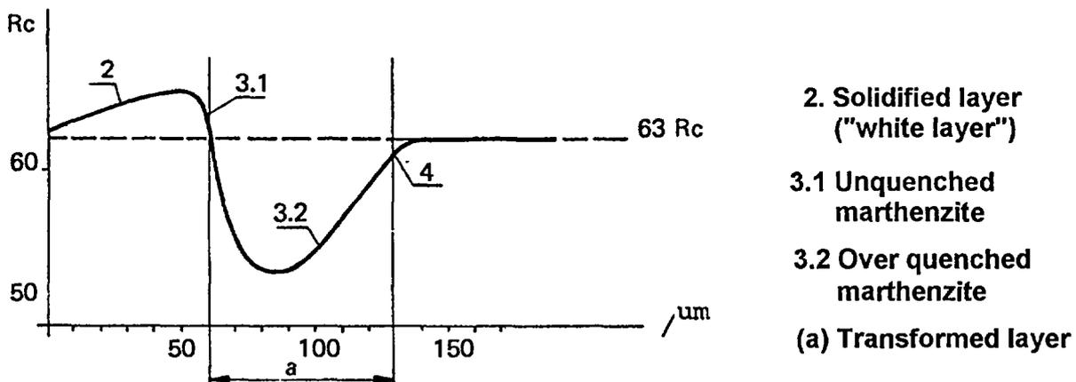
Fig. 4. Hardness profile at surface after EDM, steel Č 3840
