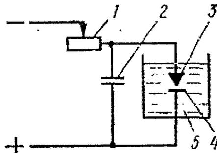
Fig. 1. Scetch of equipment for electrical discharge machining
