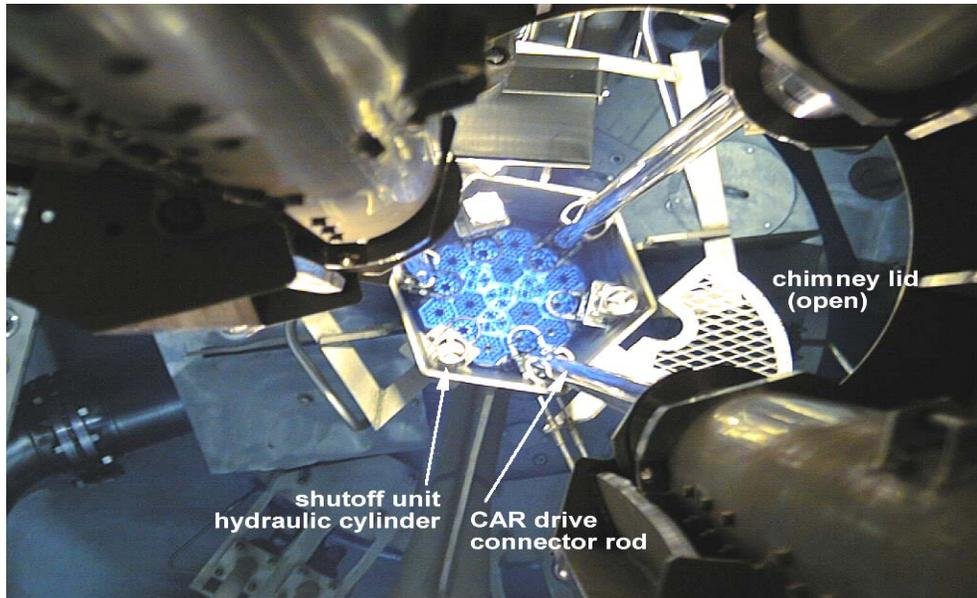
Figure 3: MAPLE Reactor Core (CAR = Control Absorber Rod)
