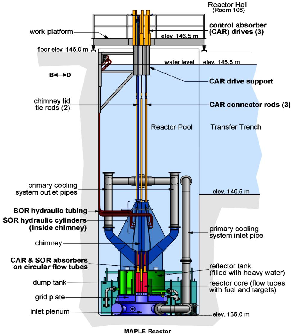
Figure 2: MAPLE Reactors (SOR = Shut-off Rod, CAR = Control Absorber Rod)
