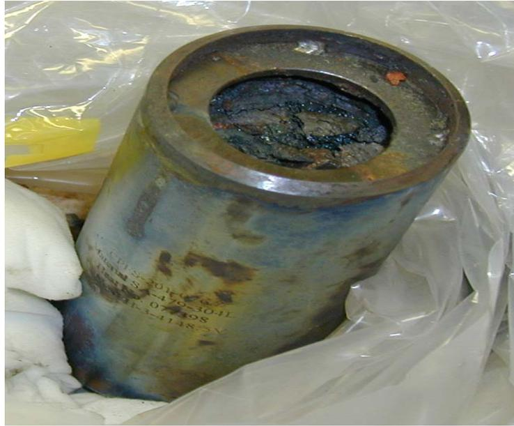
Figure 5: Calcined Uranium Waste Can
