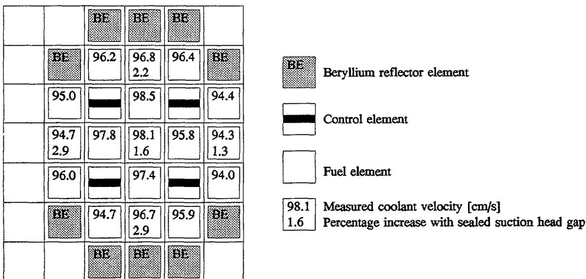
Figure 3. Coolant velocity distribution
