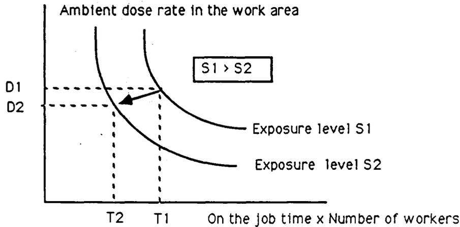
**FIG.1. Impacts of robotics and remote tooling on basic parameters governing occupational exposures at nuclear facilities.**
