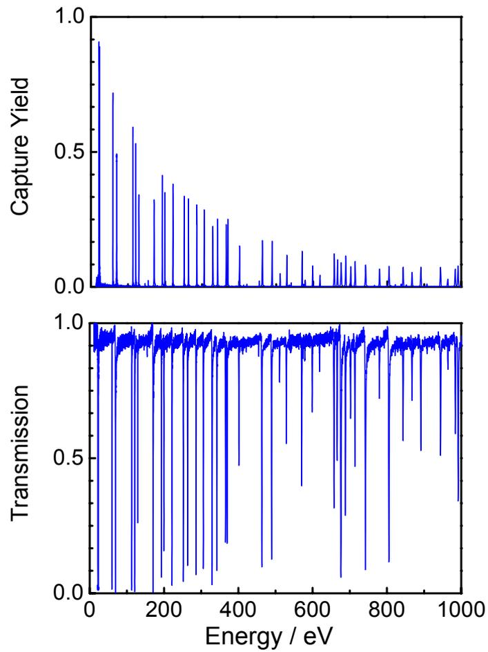
Fig.1 A comparison of the capture yield (top) and the transmission (bottom) of  $^{232}\text{Th}$  in the resolved resonance region up to 1000 eV.
