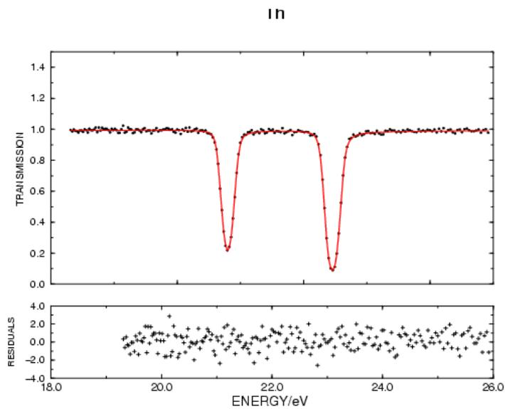
Fig. 2 The result of a renance shape analysis with REFIT\_IRMM for the 21.8 and 23.5 eV resonances of  $^{232}\text{Th}$ .
