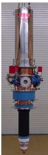
*Fig.1: Appearance of 170GHz gyrotron. Height is ~3m.*
