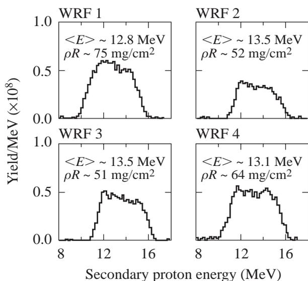
FIG. 4. Secondary proton spectra measured with four WRF spectrometers on a high-adiabat cryogenic target shot (28900). The average areal density estimated by these spectra is  $\sim 61 \pm 11 \text{ mg/cm}^2$ . One-dimensional hydrocode predictions of the capsule areal density for this shot were  $45 \text{ mg/cm}^2$ .
