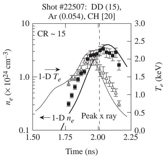
FIG. 3. Electron density and temperature as functions of time during the implosion of a 20- $\mu\text{m}$ -thick CH shell filled with 15 atm of  $\text{D}_2$  and 0.054 atm of Ar. The data for both Figs. 2 and 3 were obtained using a spectrally resolved x-ray streak camera.
