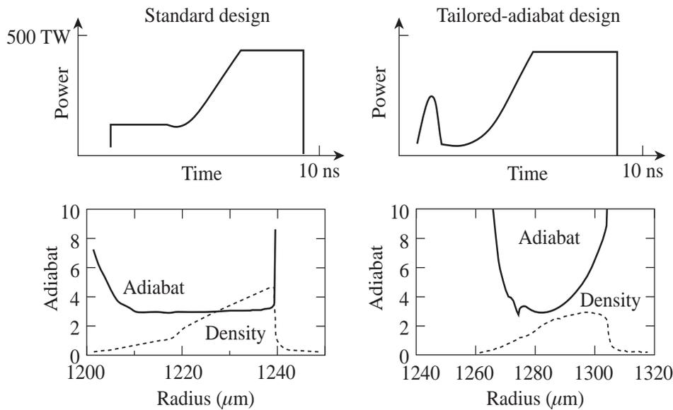
FIG. 6. Illustrations graphically demonstrating the effect of an intensity spike on the capsule implosion. The intensity spike at the leading edge of the slowly rising pulse raises the adiabat during the critical acceleration phase of the implosion for improved hydrodynamic stability but maintains a relatively low adiabat at the fuel-shell interface until late in the implosion to maximize the efficiency of the implosion.
