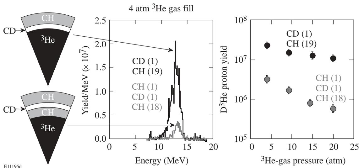
FIG. 1. Proton yield and spectrum as measured with an array of WRF spectrometers in implosions of  $^3\text{He}$ -filled (4 to 20 atm) CH shells containing a 1- $\mu\text{m}$ -thick layer of CD. On targets with a CD layer located 1  $\mu\text{m}$  away from the gas, the  $\text{D}^3\text{He}$  proton yield is less than one-tenth that of the targets with the CD layer adjacent to the  $^3\text{He}$  gas.
