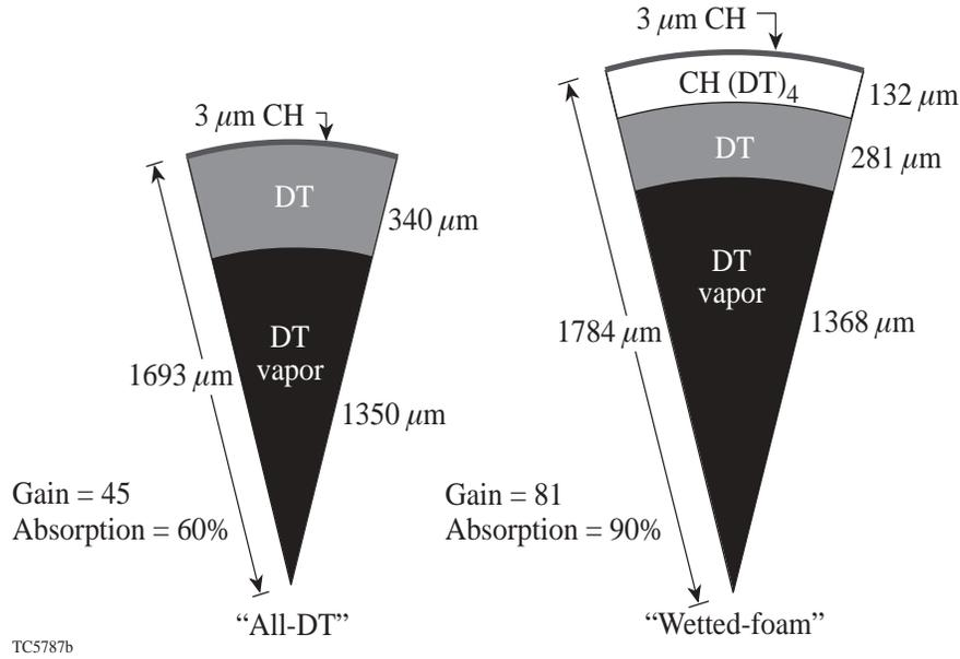
FIG. 5. Schematic representation of a base-line NIF direct-drive target (all-DT) compared to the “wetted-foam design.”
