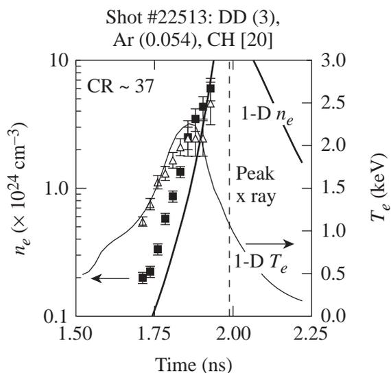
FIG. 2. Electron density and temperature as functions of time during the implosion of a 20- $\mu\text{m}$ -thick CH shell filled with 3 atm of  $\text{D}_2$  and 0.054 atm of Ar. The triangles (electron temperature) and squares (electron density) indicate the experimental measurements inferred from time-resolved Ar spectroscopy; the solid lines represent the 1-D hydrodynamic code predictions.
