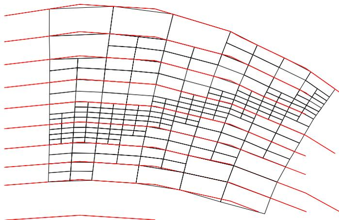
*Fig. 6 Parent grid adapted to the moved front*
