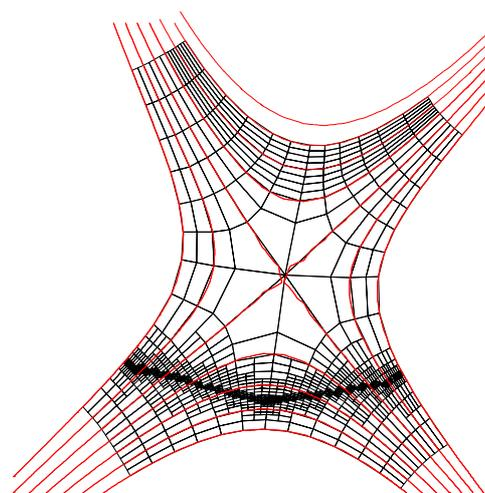
*Fig. 2 Aligned and adapted grid near the X-Point*
