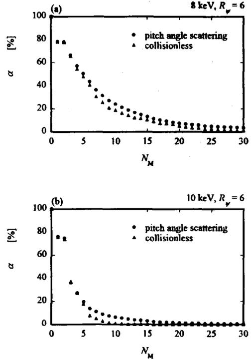
FIG. 12. Relation between confined fast ion fraction in percentage and the number of mirror reflection. Injection beam energies are (a) 8 keV and (b) 10 keV, and the mirror ratio is  $R_p = 6$  for both (a) and (b).
