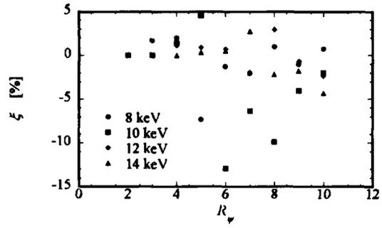
FIG. 11. The mirror ratio dependence of total deposition power increment (decrement)  $\xi$  due to pitch angle collisions for the injected beam energy of 8 keV (solid circle), 10 keV (solid square), 12 keV (solid diamond), and 14 keV (solid triangle).
