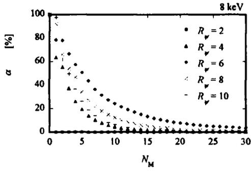
FIG. 9. Relation between confined fast ion fraction in percentage and the number of mirror reflection. Injection beam energy is 8 keV here. The values of mirror ratio control parameter  $R_p$  are 2 (solid circle), 4 (solid triangle), 6 (solid diamond), 8 (cross), and 10 (plus).
