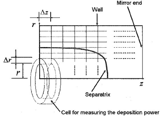
FIG. 5. Schematic drawing of simulation space
