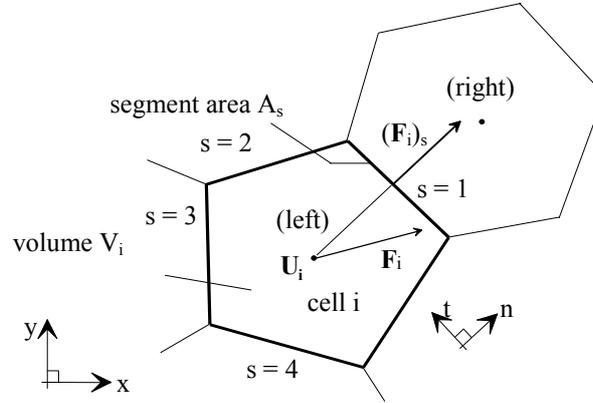
**Figure 3:** Finite volume discretization
