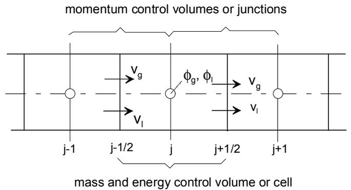
**Figure 1:** Space discretization for one-dimensional flow
