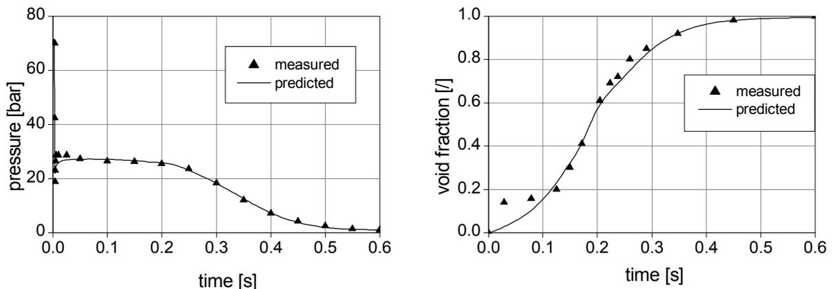
**Figure 6 :** Pressure at pipe head and void fraction at pipe middle section
