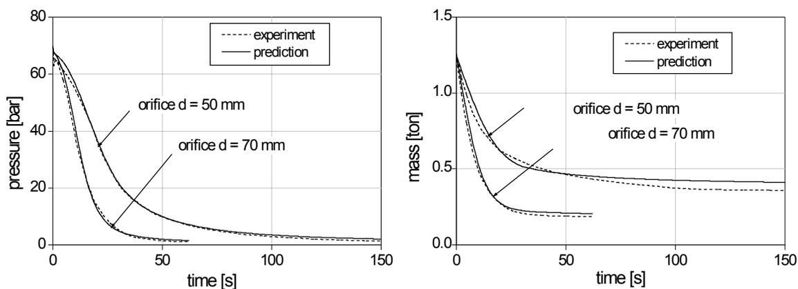
**Figure 8:** ROSA-I vessel blowdown, comparison of measured and predicted pressure and mass inventory for two different break sizes
