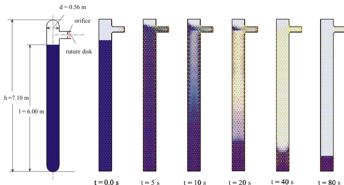
**Figure 7:** ROSA-I vessel blowdown, predicted void fraction and flow vector fields at different time values.
