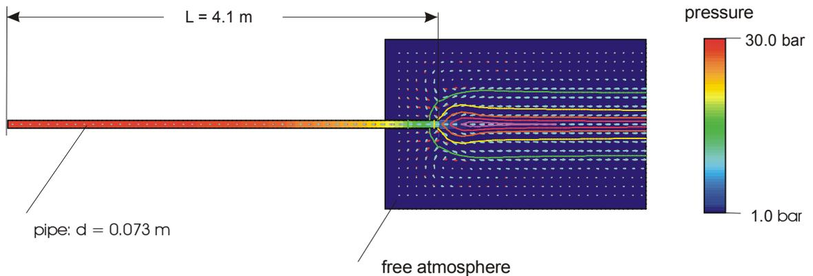
**Figure 5:** Pressure distribution and iso-Mach lines at  $t = 0.02$  s after break
