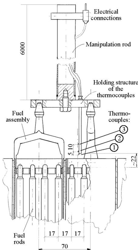
**Figure 1:** Structure and position of the measuring equipment at the top of the fuel assemblies
