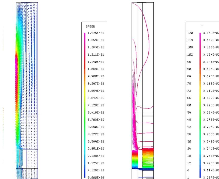
**Figure 5:** Velocity and temperature field 4 hours after start-up
