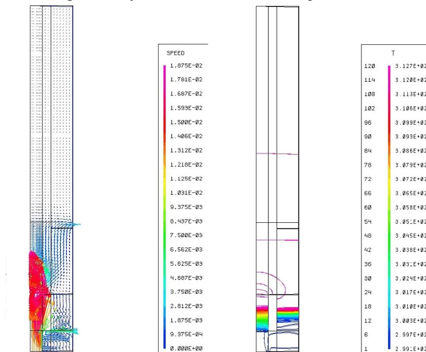
**Figure 4:** Velocity and temperature field 3 hours after start-up
