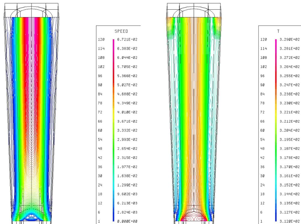
**Figure 6:** Velocity and temperature field above a fuel element
