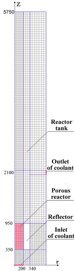
**Figure 3:** Geometry model for 2D computations
