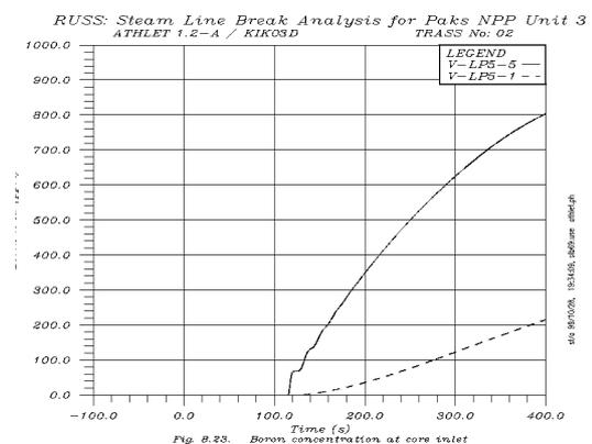
Fig.9: Core inlet boron concentration
