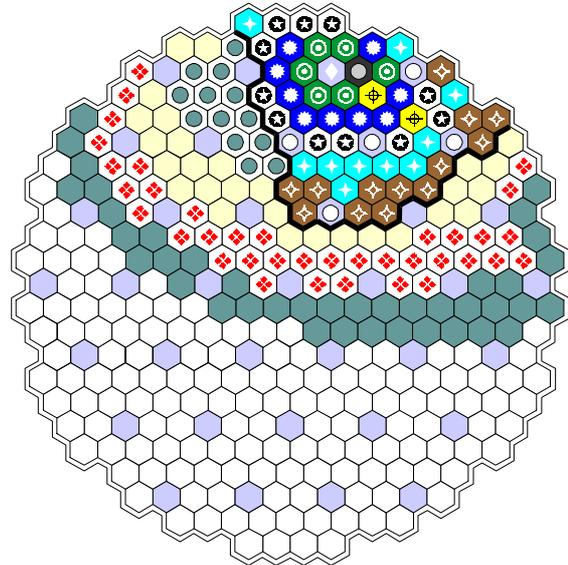
**Fig. 1:** Nodalization of the core into super-channels
