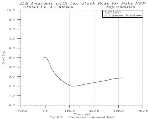
**Fig.18 :** Pressuriser collapsed level
