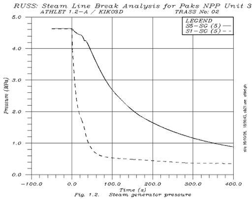
Fig.4: Pressure of the steam-generators
