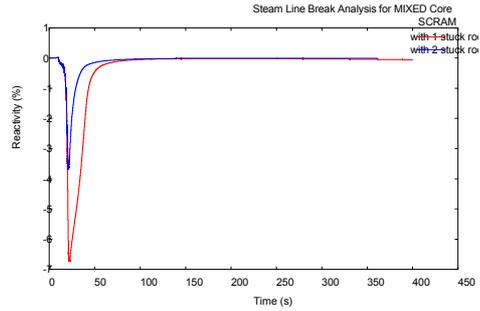
**Fig. 13:** The Reactivity of the core during MSLB, calculated for the two type of SCRAM
