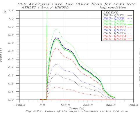
**Fig.19 :** Assembly power in various super-channel
