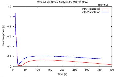
**Fig. 12:** The Relative Core Power during MSLB, calculated for the two types of SCRAM
