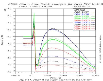
Fig.10: Assembly power in various super-channels
