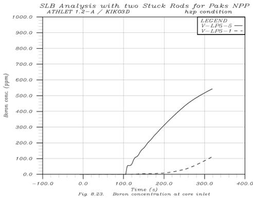
**Fig.16 :** Core inlet boron concentration
