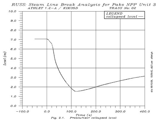
Fig.8: Pressuriser collapsed level
