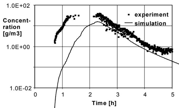
**Figure 5.** Total wet aerosol mass concentration in test vessel (test K186)
