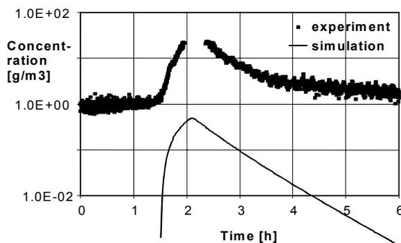
**Figure 11.** Total wet aerosol mass concentration in test vessel (test K148)
