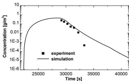
**Figure 2.** Total dry aerosol mass concentration in test vessel (test K188)
