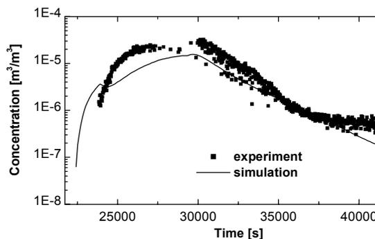
**Figure 3.** Total wet aerosol volumetric concentration in test vessel (test K188)
