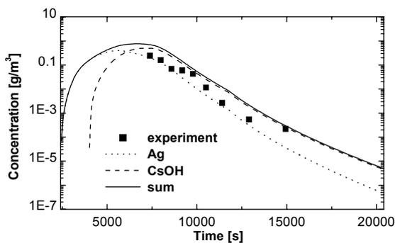
**Figure 4.** Total dry aerosol mass concentration in test vessel (test K186)
