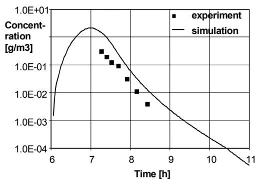
**Figure 6.** Total dry aerosol mass concentration in test vessel (test K187)
