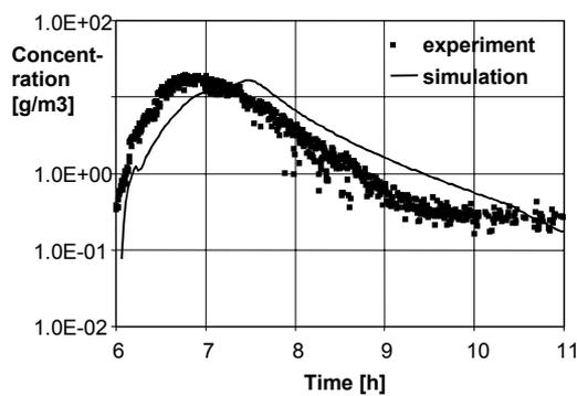
**Figure 7.** Total wet aerosol mass concentration in test vessel (test K187)
