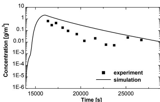
**Figure 8.** Total dry aerosol mass concentration in test vessel (test K123)
