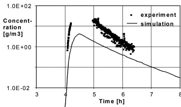
**Figure 9.** Total wet aerosol mass concentration in test vessel (test K123)
