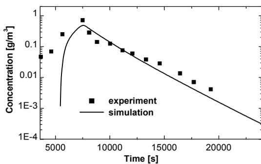
**Figure 10.** Total dry aerosol mass concentration in test vessel (test K148)
