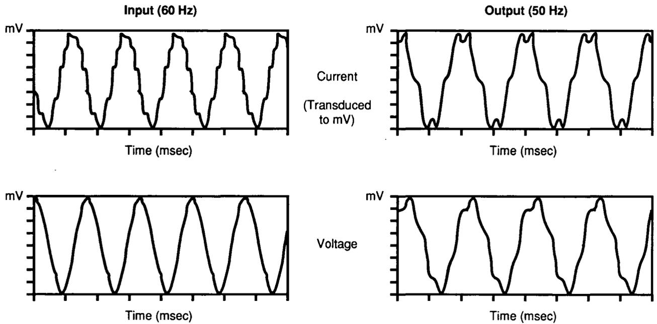
Figure 3. Voltage and Current GTO Inputs and Outputs
