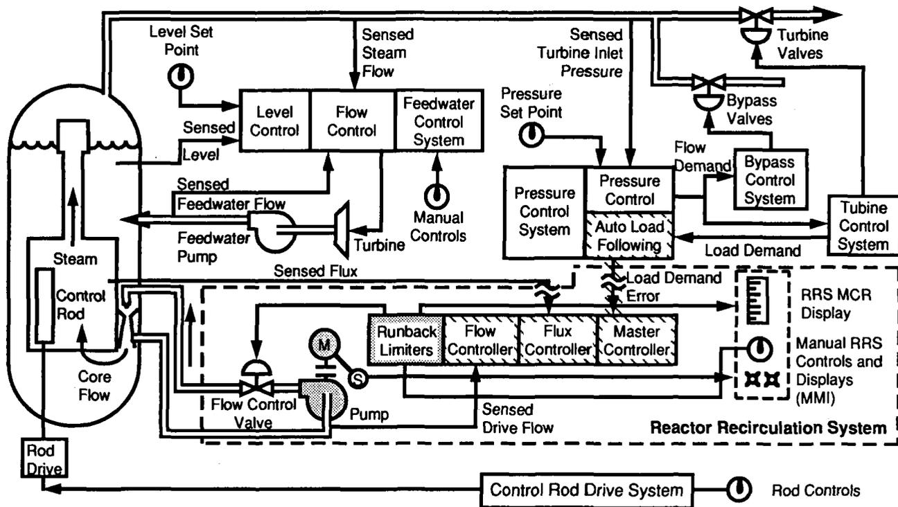
Figure 5. BWR 5/6 Flow Control Valve Configuration
