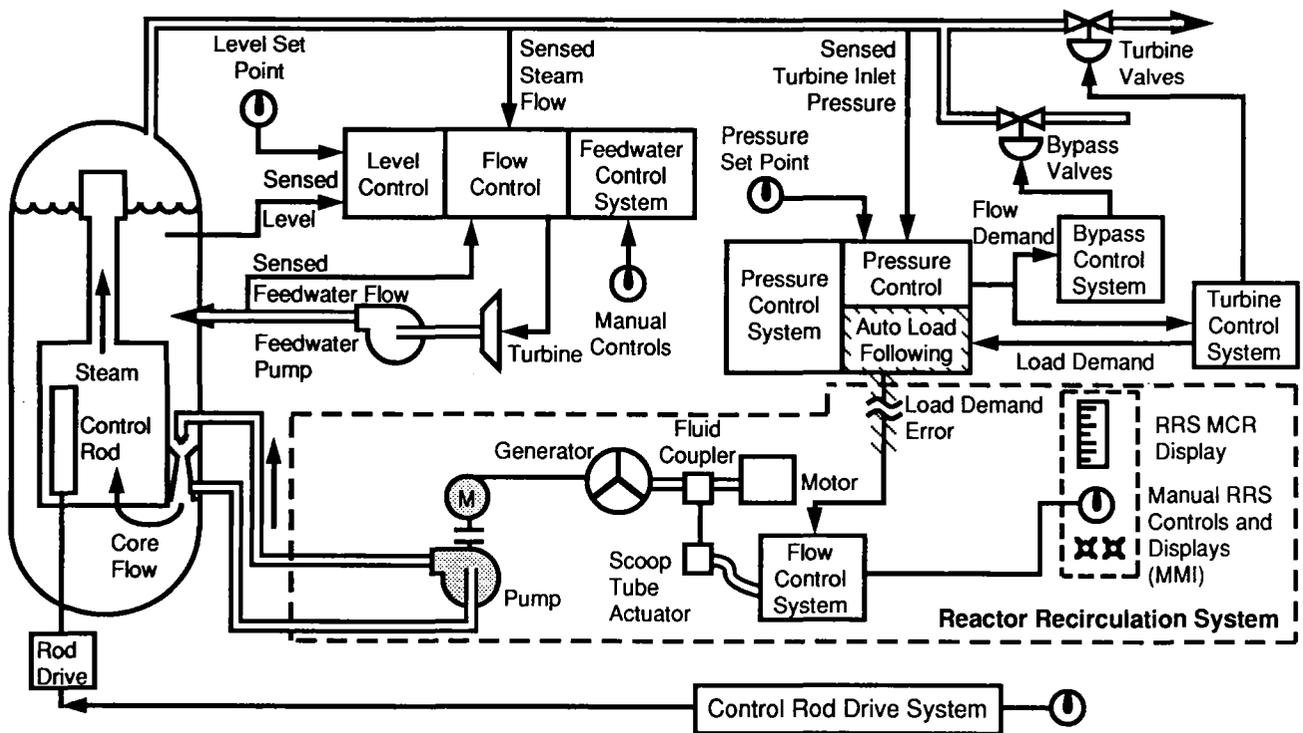
Figure 4. BWR 3/4 MG Set Configuration
