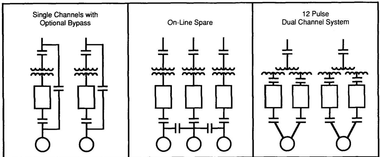
Figure 1. ASD System Configurations
