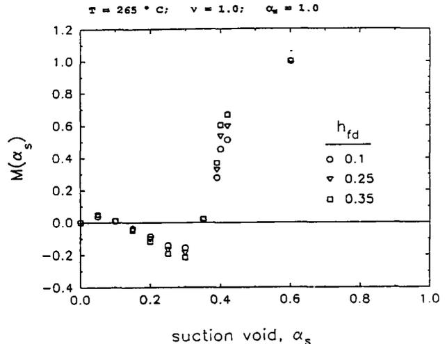
FIGURE 8: SENSITIVITY OF  $M(\alpha)$  TO  $h_{fd}$  VALUES
