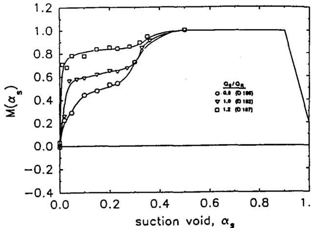
FIGURE 7: HEAD DEGRADATION MULTIPLIER (T = 200 deg C)
