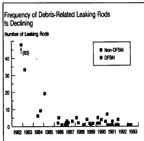
Power plant operators have also made a significant impact in the occurrence of debris related fuel leakage, due to their increased sensitivity to "good housekeeping" and improved machining operations. With the introduction of PERFORMANCE+ fuel, Westinghouse has extended debris protection to include two additional levels. The first of these PERFORMANCE+ features is the protective grid which is illustrated in Figure
