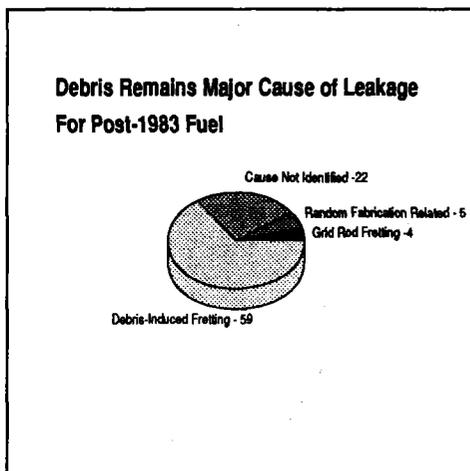
As illustrated, the single largest fuel rod leakage mechanism has been debris-induced fuel rod freting. The freting is
