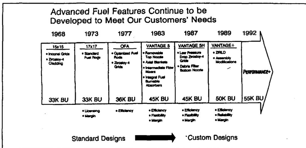
ratepayers. Advanced product development has been a continuous process at Westinghouse responding to the electric utility's needs for improved fuel cycle cost, zero-defect reliability, extended cycle lengths and ultra-high discharge burnup. Figure 1 illustrates the continuous fuel product development at Westinghouse since the early 1970s.
