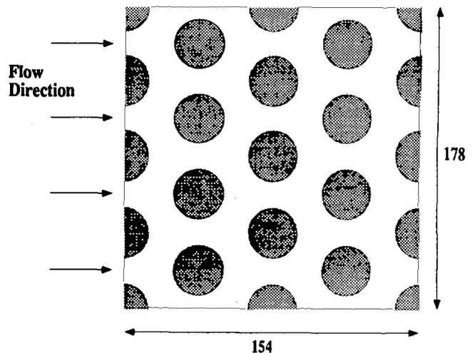
Figure 2: Geometry for triangular pitch deep bundle
