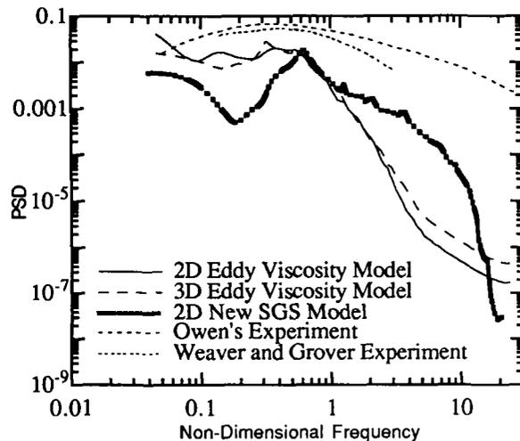
Figure 4: Normalized one-dimensional power spectrum for turbulent triangular bundle flow. Abscissa is given by  $[(fd/U_g)(L/d)(T/d)]$
