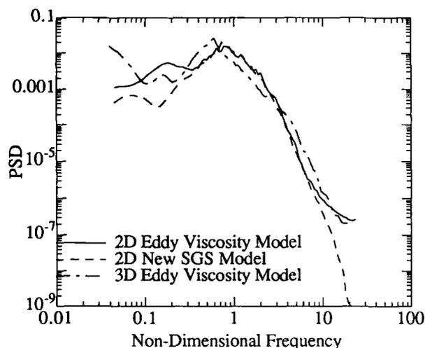
Figure 5: Normalized power spectrum of the drag coefficient for turbulent triangular bundle flow. Abscissa is given by  $[(fd/U_g)(L/d)(T/d)]$
