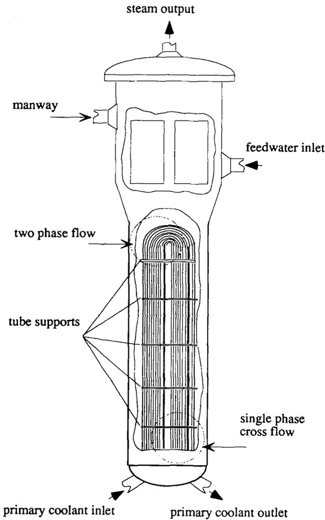
Figure 1: U-tube steam generator
