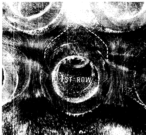
Photo 3 Flow pattern of Re_{max}=7540 at the first row in the tube bank of P/d=1.33 .
