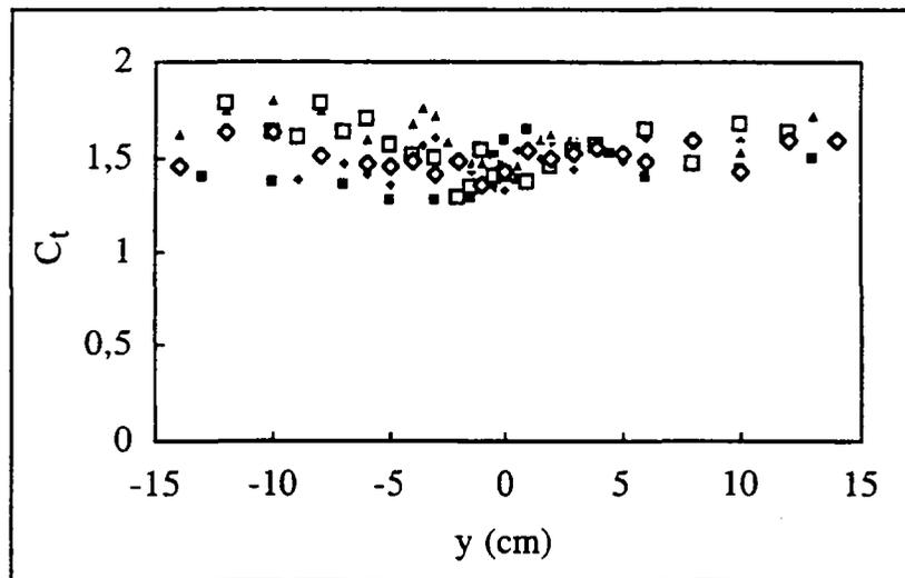
Figure 6 :Dimensionless longitudinal velocity fluctuations in gas phase:  $C_t = u'_G/u'_L$ . Transverse profiles at different longitudinal sections in bubbly mixing layer (from  $x = 6$  cm to  $x = 50$  cm).
