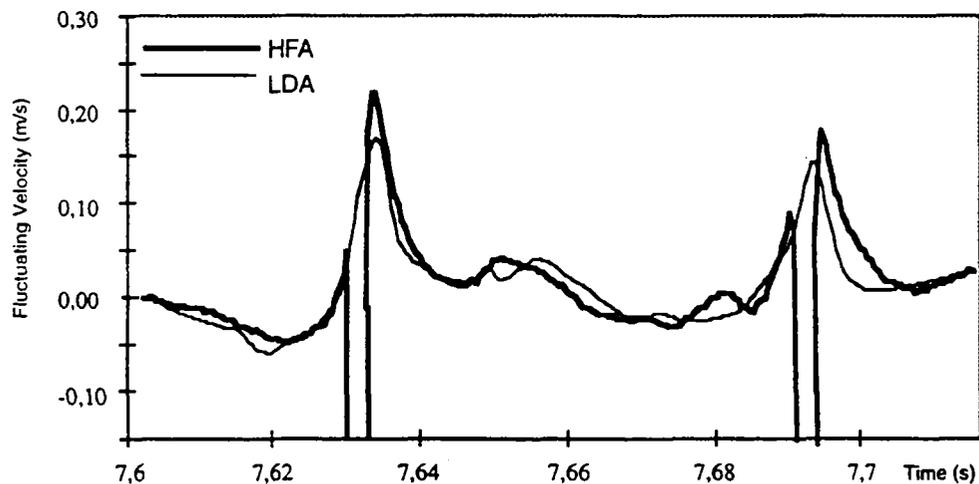
*Figure 1: Untreated HFA - LDA after treatment in bubbly flow ( $\alpha = 1\%$ ,  $d_b = 2.5$  mm).*
