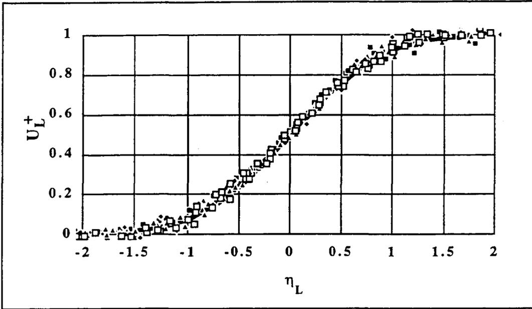
Figure 2 : Dimensionless mean velocity distributions in liquid phase in single-phase (solid symbols  $\sigma = 24$ ) and in bubbly mixing layer (open symbols  $\sigma = 11$ ) and Goertler law (solid line). ( $U^+ = (U - U_1) / \Delta U$ ,  $\eta = \sigma y / x$ )
