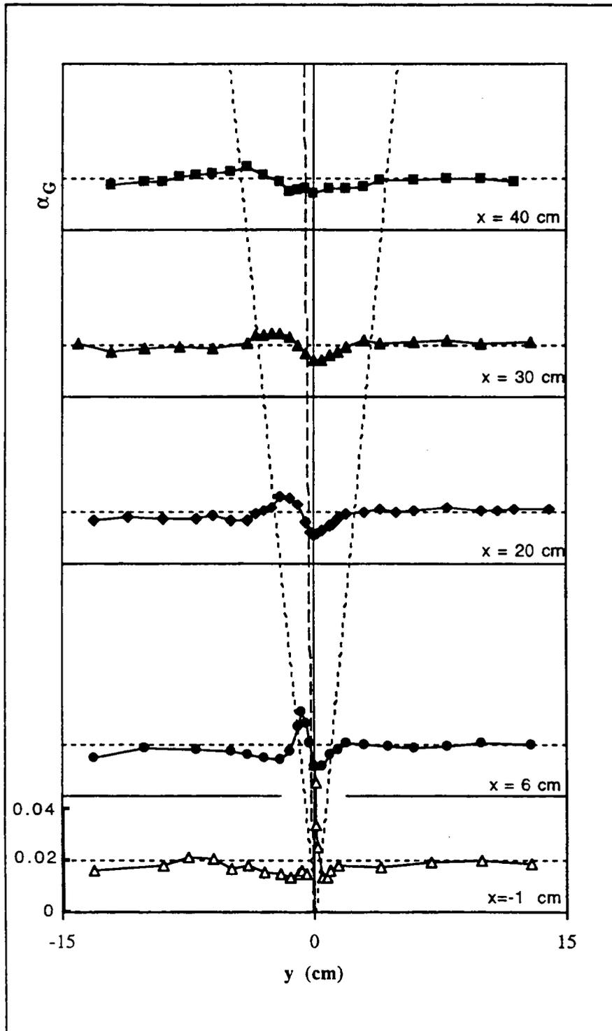
Figure 4 : Transverse Void fraction profiles at different longitudinal sections in bubbly mixing layer (y=0, axe of 20 cm x 20 cm square vertical channel)
