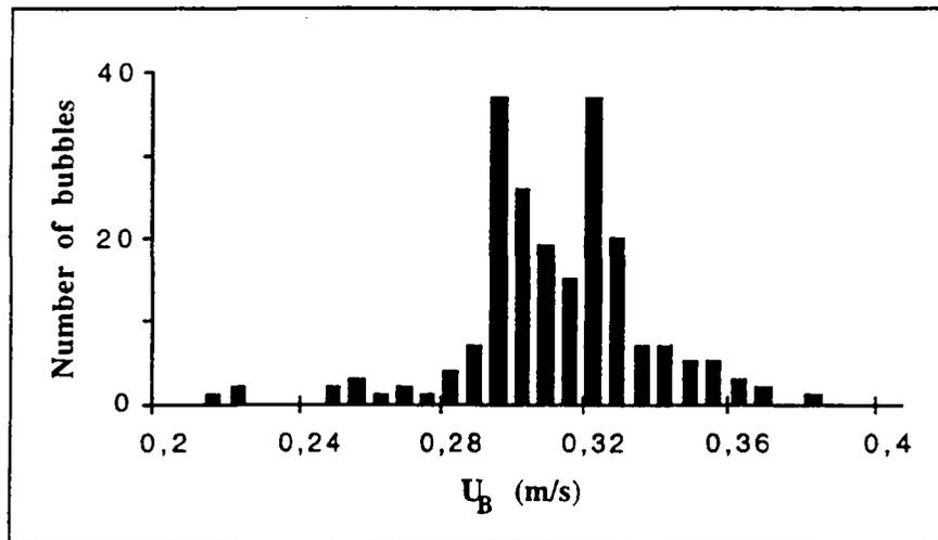
Figure 5: Bubble velocity histogram in stagnant water (Mean associated bubble chord: 1,8 mm)
