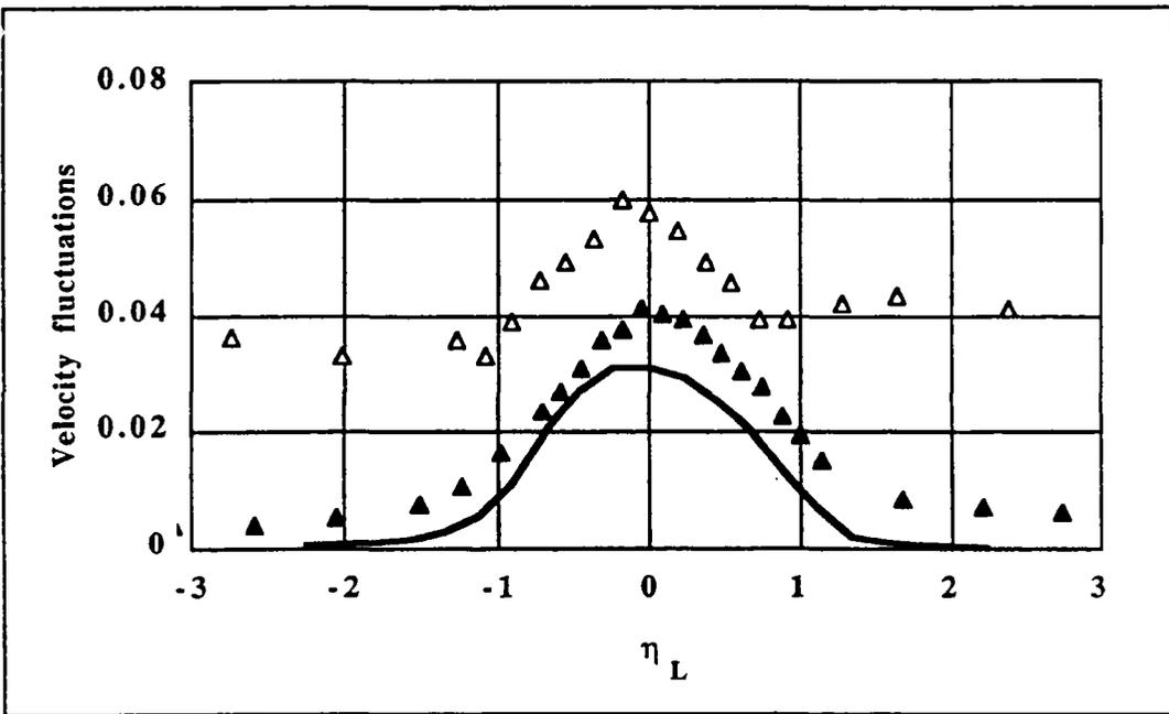
Figure 3 : Dimensionless longitudinal turbulent velocity fluctuations in liquid:  $u'^2 / \Delta U^2$
