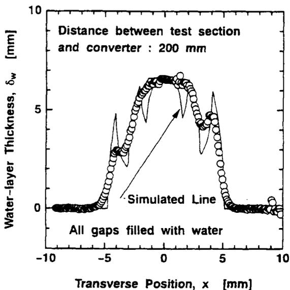
Fig.12 Effect of the distance between the test section and the converter on the water-layer thickness profile measured by the  $\Sigma$ -scaling method.
