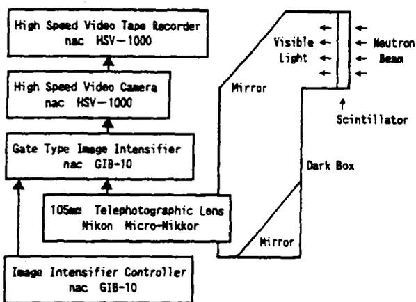
Fig.2 Block diagram of the imaging system for high-frame-rate NR with a steady neutron beam.
