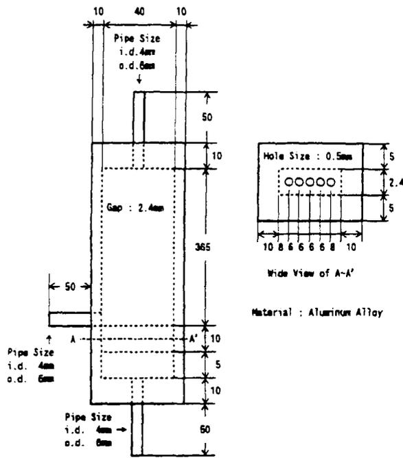
Fig.3 Schematic drawing of the test section used in the two-phase flow experiment.
