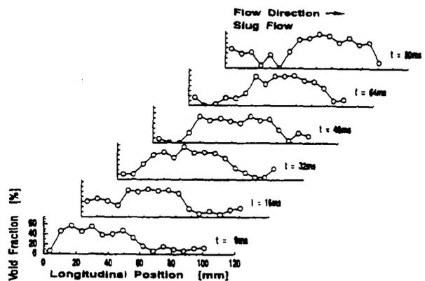
Fig.14 Temporal variation of void profile in slug flow along the flow direction.
