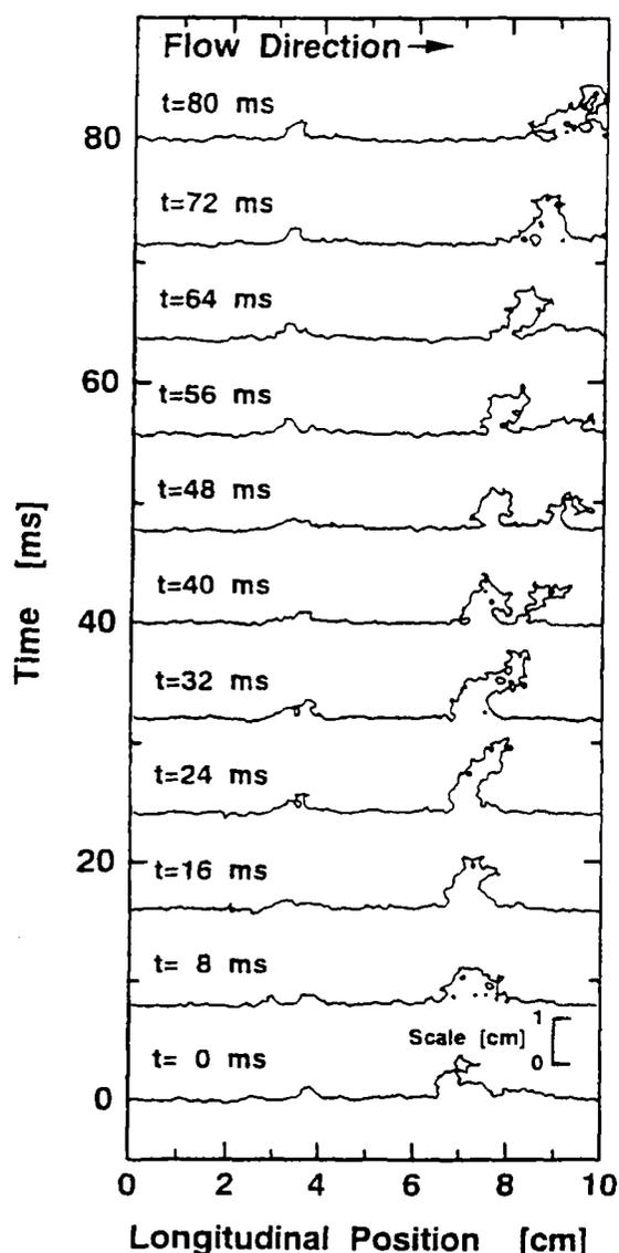
Fig.10 Motion of a disturbance wave on the annular liquid film depicted by image processing (edge detection).
