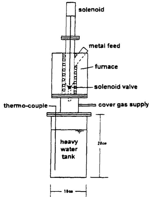
Fig.4 Test rig for the molten-metal-water interaction experiment.
