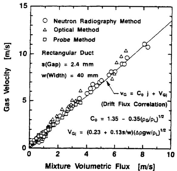
Fig.13 Comparison of the measured void fractions taken by the real-time NR, optical and conductance methods with the drift flux correlation.
