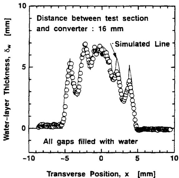
Fig.11 Comparison between the designed and measured profiles of water thickness for the triple tube test section with all the gaps filled with water.
