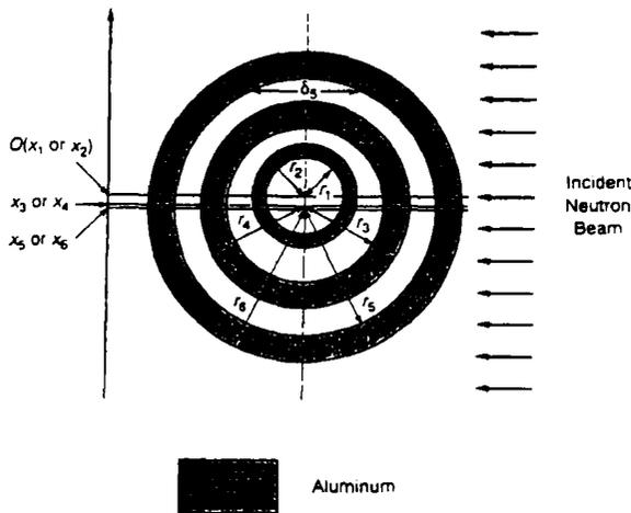
Fig.5 Cross sectional view of the triple tube test section.
