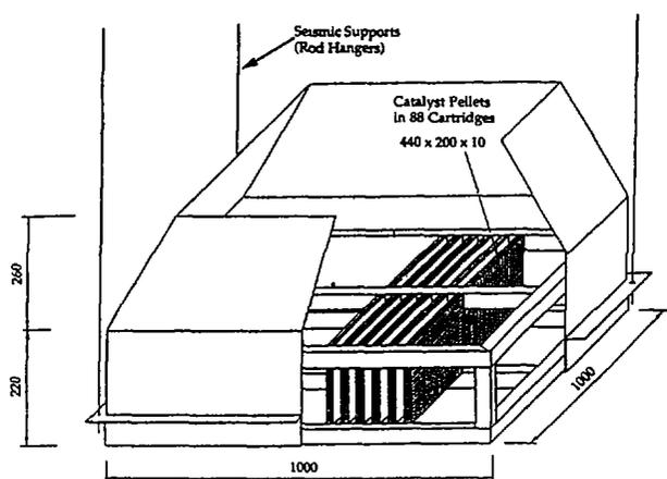
Figure 1 - Drawing of the Prototype PAR Device (Dimensions are in cm.)
