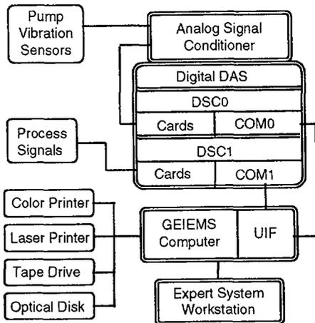
Figure 1a GEIEMS/Expert System Block Diagram with Conventional Digital DAS
