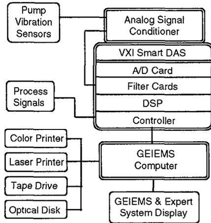
Figure 1b GEIEMS/Expert System Block Diagram with VXI Type Smart DAS
