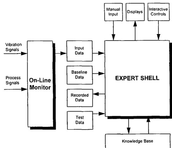
Figure 2 Expert System Interface Diagram
