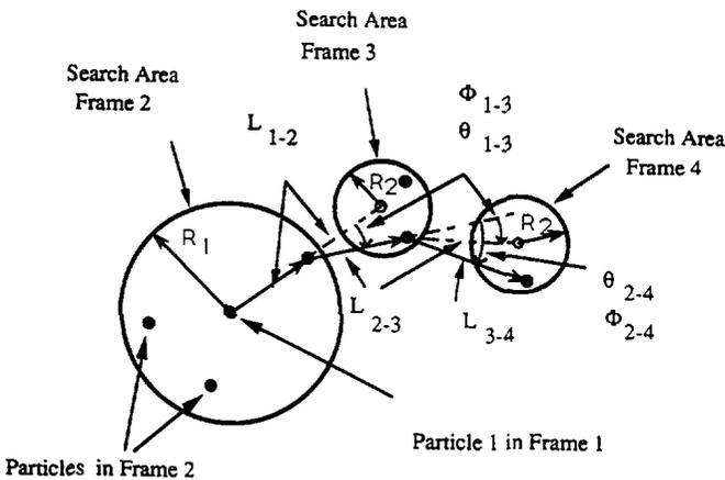
Figure 2: Description of the Multiframe Tracking Technique
