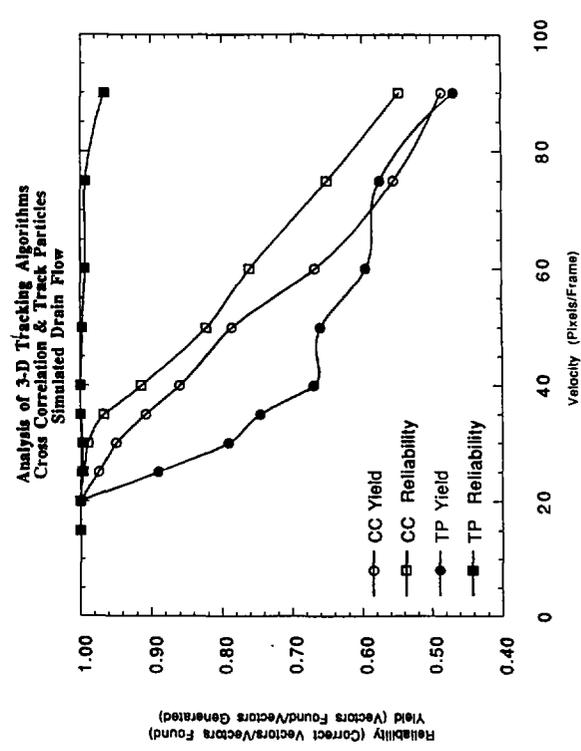
Figure 11: Analysis of 3D Tracking Algorithms Cross Correlation and Track Particles for Simulated Drain Flow
