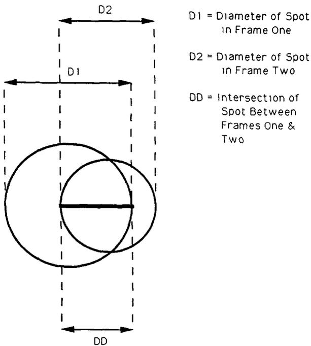
Figure 3: Intersection of Spot i Between Frames 1 and 2
