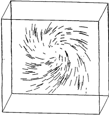
Figure 8: Output from Multiframe Tracking Code (synthetic drain flow, 4 frames, 200 particles, 30 pixels/frame) Top View (into drain)
