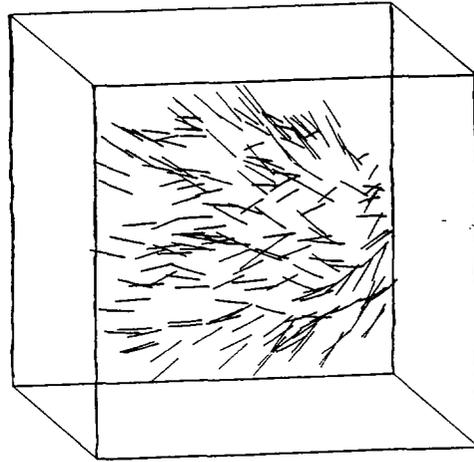
Figure 9: Output from Multiframe Tracking Code (synthetic drain flow, 4 frames, 200 particles, 30 pixels/frame) Side View
