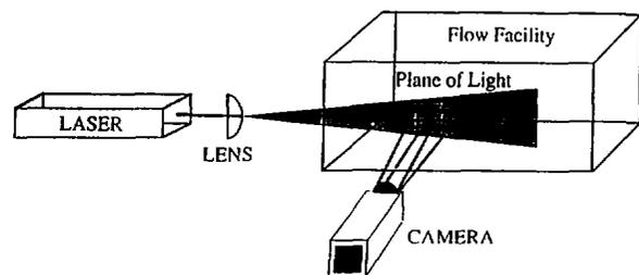
Figure 1: Two-Dimensional PIV Setup
