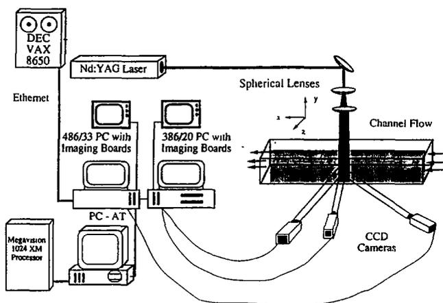
Figure 12: Three-Dimensional PIV Experimental Setup
