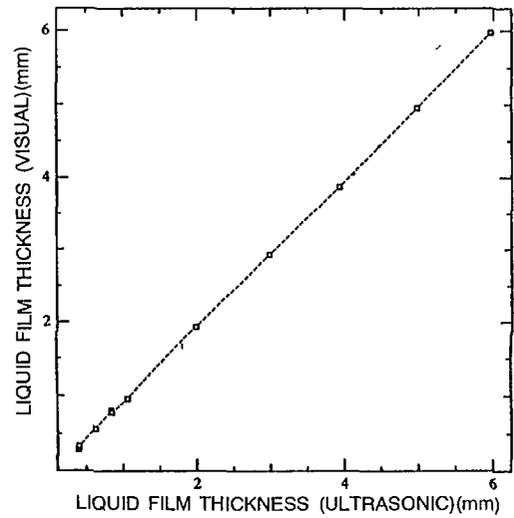
Fig.3 Comparison of the results obtained by ultrasonic transmission technique and by visualization in still water
