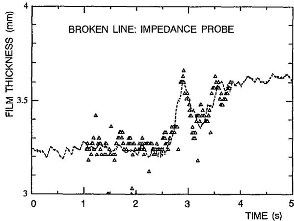
Fig.11 Comparison of the ultrasonic transmission technique with impedance probe method
