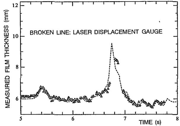
Fig.7 Comparison of the ultrasonic transmission technique with laser technique for standing wave
