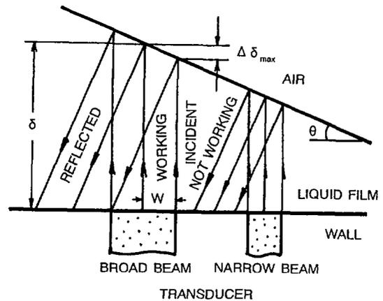
Fig.12 Sensitivity to the inclination angle of the reflection interface
