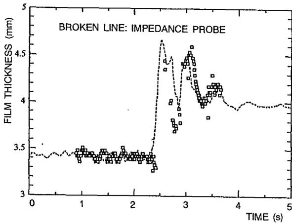
Fig.10 Comparison of the ultrasonic transmission technique with impedance probe method
