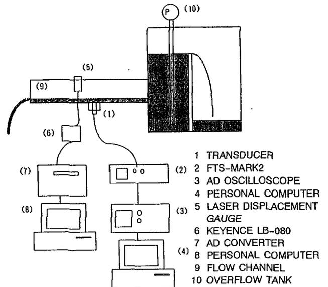
Fig.4 A schematic of the flow test section and measurement arrangement
