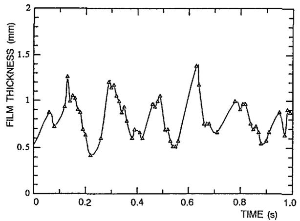
Fig.8 Time-dependent film thickness in stratified flow
