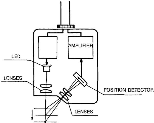
Fig.5 Operational principle of a laser displacement gauge
