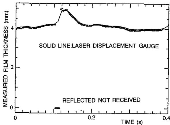
Fig.6 Comparison of the ultrasonic transmission technique with laser technique for standing wave
