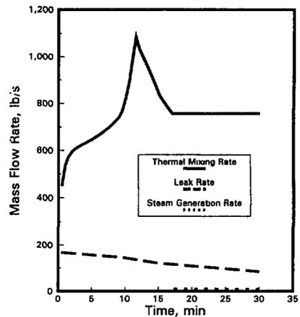
Figure 3c - Mass Flow Rates Following Loss of RHR in the Presence of Inadvertent Leakage and Partial Injection ( $\dot{V}_{inj} = 100 \text{ gpm}$ ).
