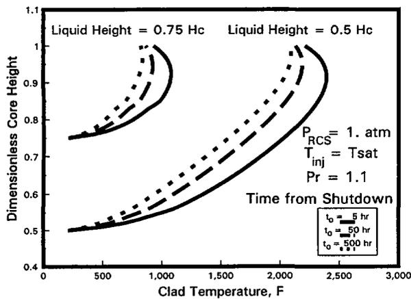
Figure 2d - Clad Temperature Distribution in the Uncovered Core as a Function of Collapsed Liquid Height and Time From Reactor Shutdown ( $T_{inj} = T_{sat}$ ).
