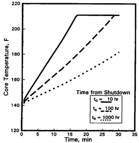
Figure 3a - Temperature Response of BWR Water Inventory to Loss of RHR, Inadvertent Leakage, and Partial Injection ( $\dot{V}_{inj} = 100 \text{ gpm}$ ).
