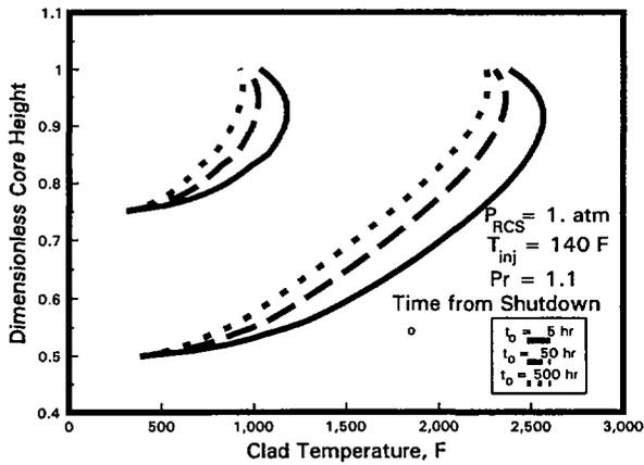
Figure 2c - Clad Temperature Distribution in the Uncovered Core as a Function of Collapsed Liquid Height and Time From Reactor Shutdown ( $T_{inj} = 140 \text{ }^\circ\text{F}$ ).
