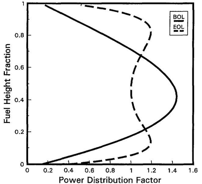
Figure 2a - Axial Power Distributions for Beginning and End of Life.
