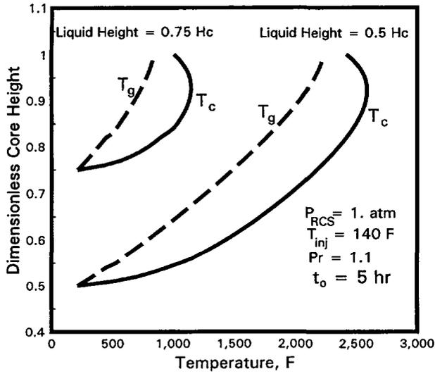
Figure 2b - Axial Temperature Distributions for Clad ( $T_c$ ) and Flowing Steam ( $T_g$ ) in the Uncovered Core.
