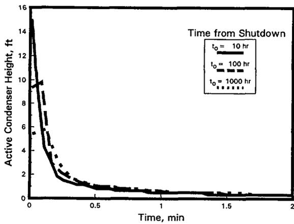
Figure 1c - Active Condenser Height During Establishment of Reflux Cooling ( $n_{sg} = 4$ ).
