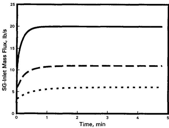
Figure 1b - SG Inlet Mass Flow Rates During Establishment of Reflux Cooling ( $n_{sg} = 4$ ).
