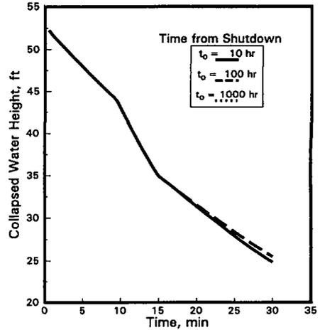
Figure 3b - Response of Collapsed Water Level to Loss of RHR in the Presence of Inadvertent Leakage and Partial Injection ( $\dot{V}_{inj} = 100 \text{ gpm}$ ).
