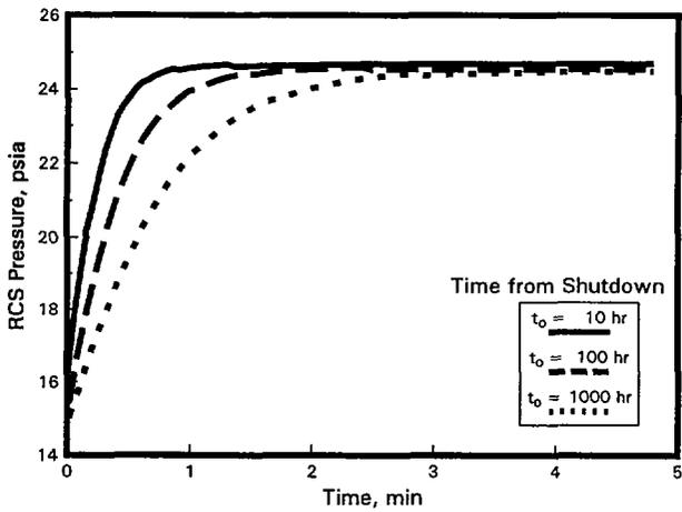
Figure 1a - RCS Pressure Response to Establishment of Reflux Cooling ( $n_{sg} = 4$ ).
