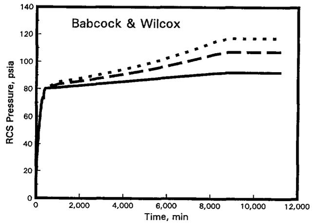
Figure 1d - Effects of Humidification Extent for Accumulated Air on RCS Pressure Response to Reflux Cooling.
