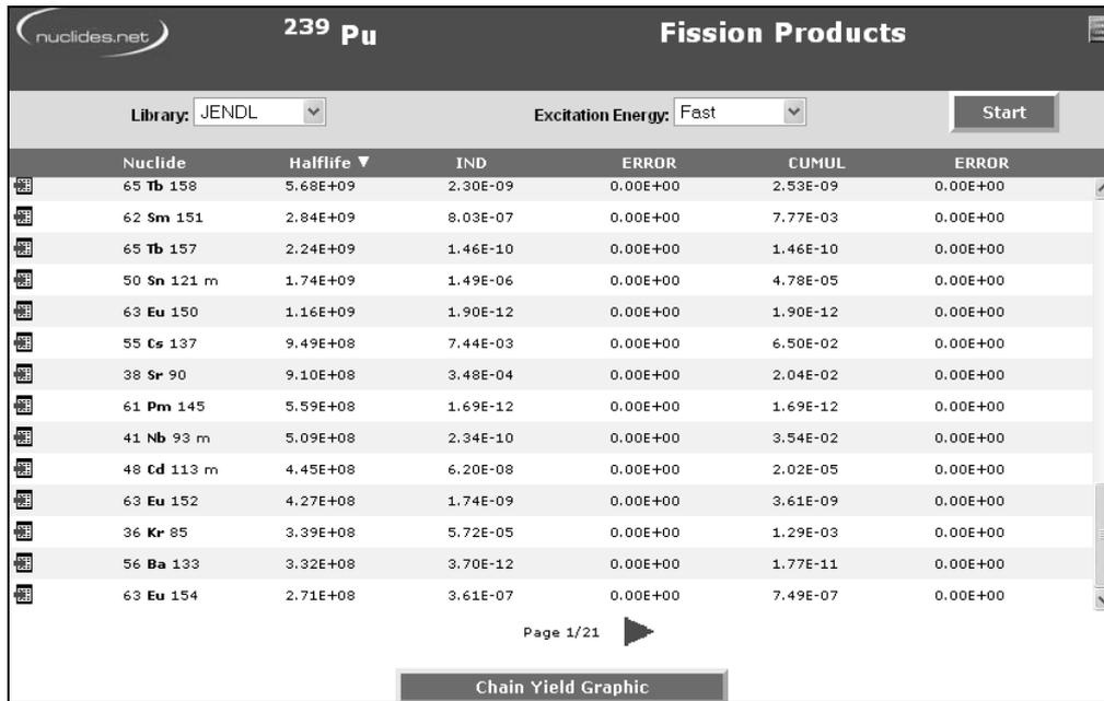
Figure 1: Fission yield module for the <sup>239</sup>Pu fission with fast neutrons
