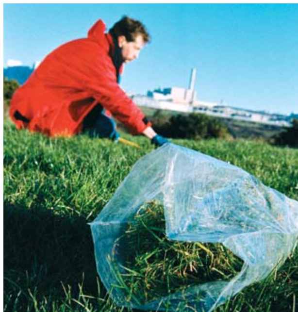
Environmental monitoring: taking samples of grasses near the COGEMA-La Hague used fuel treatment plant (Cherbourg, France).
