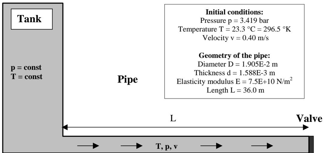
*Figure 2: Geometry and initial conditions of Simpson's experiment*
