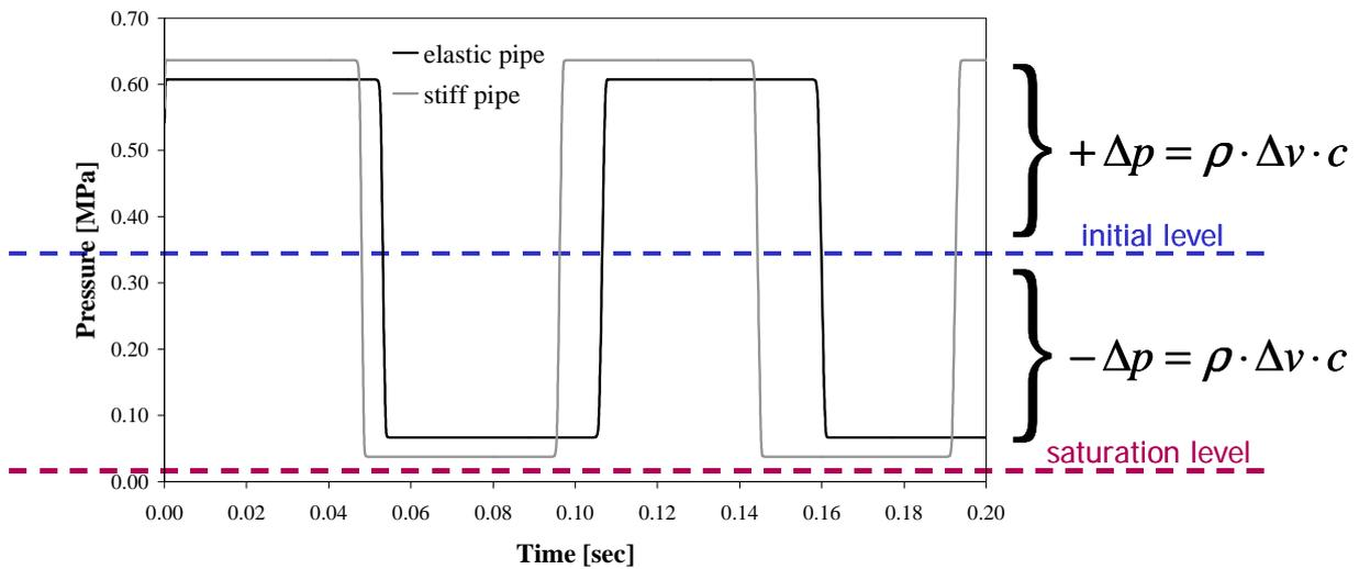
**Figure 3:** Pressure history near the valve – no flashing ( $v_0 = 0.20$  m/s)
