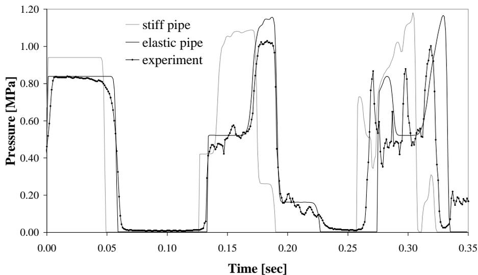
**Figure 4:** Pressure history near the valve – flashing ( $v_0 = 0.40$  m/s)
