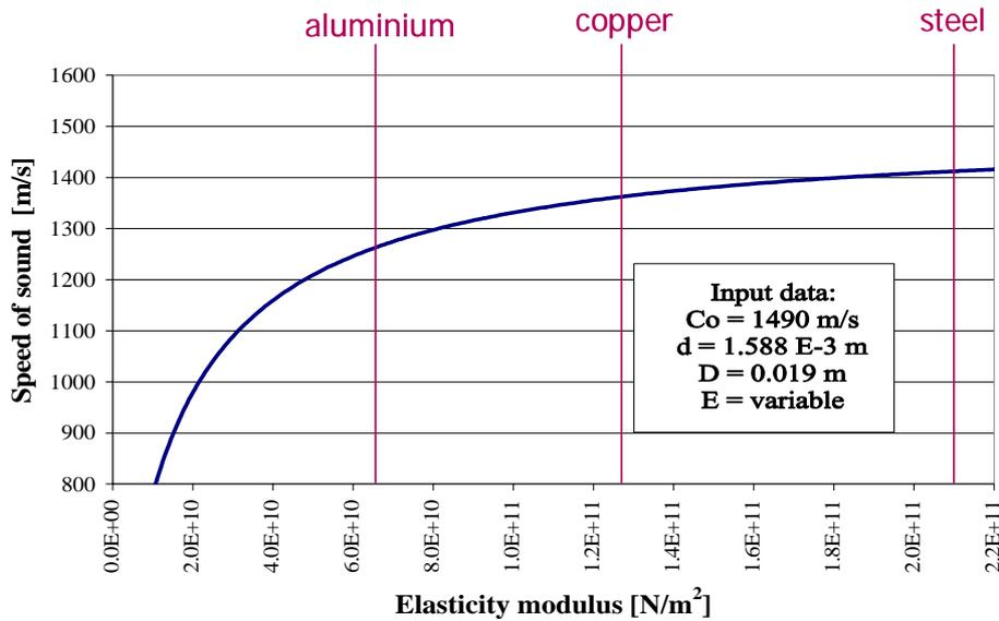
**Figure 1:** Speed of sound - dependency on Elasticity modulus
