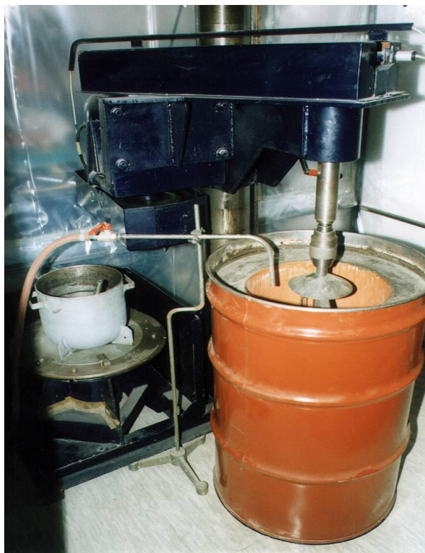
Figure 1: Modified pilot mixer with concrete container made in metal barrel
