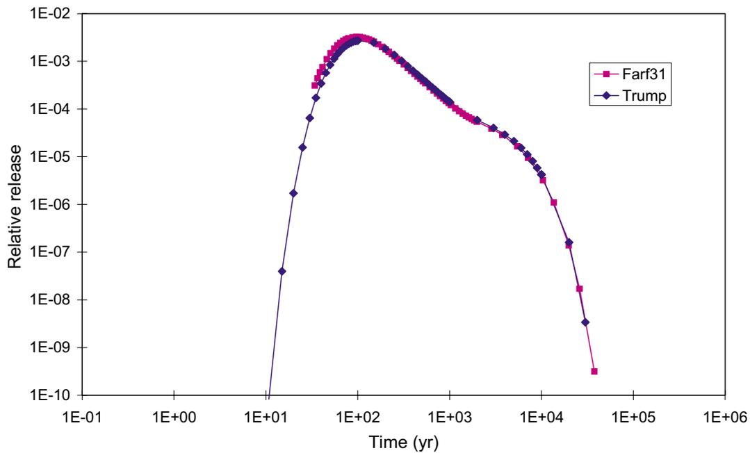
*Figure 4-7. Comparison of the response function from FARF31 and the numerical model TRUMP.*
