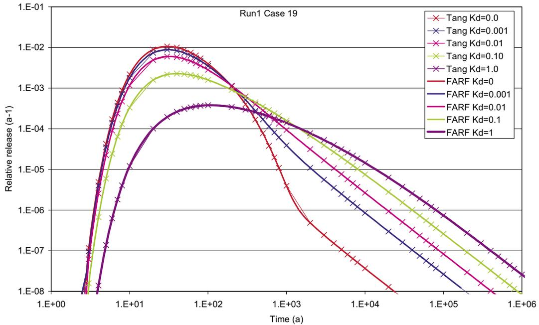
**Figure 4-4.** Comparison of Tang solution of the advection dispersion equation with matrix diffusion and sorption and results from FARF31. Case D.
