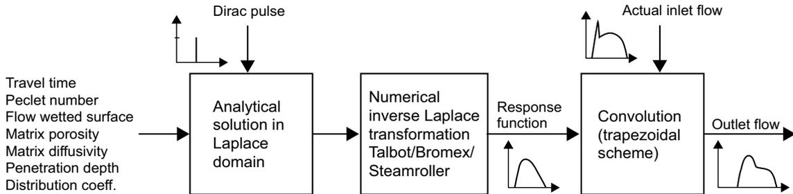
**Figure 3-1.** Schematic illustration of the solution technique used in FARF31.
