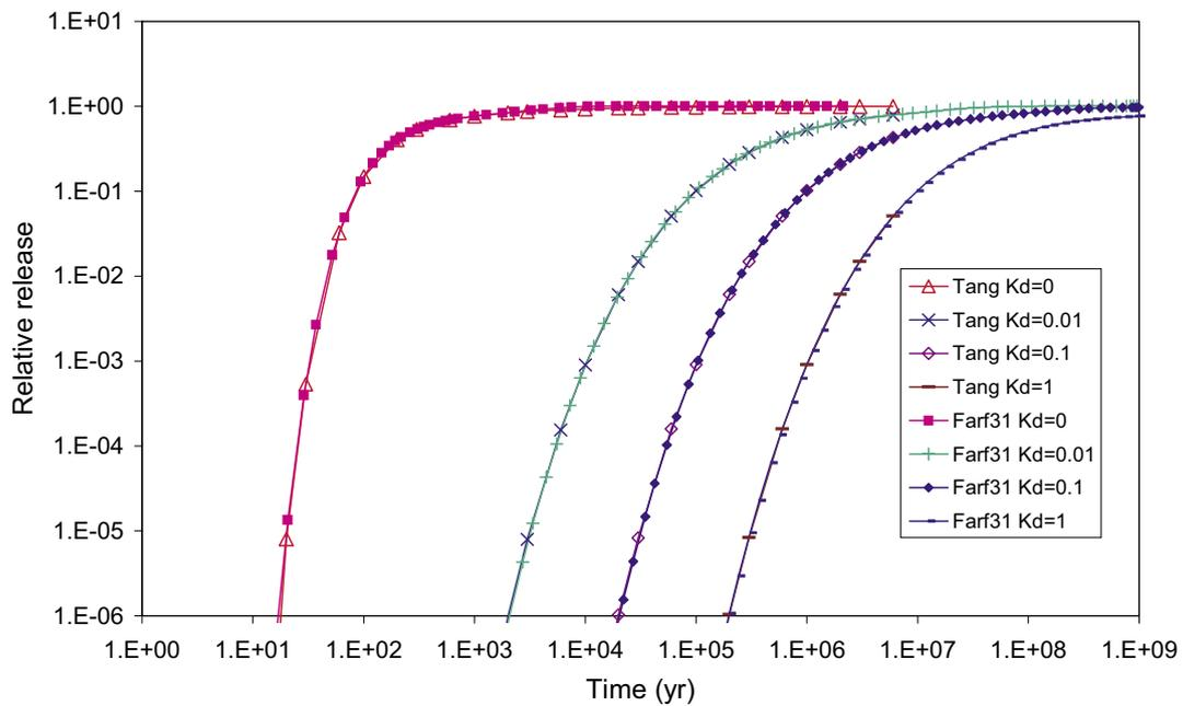
**Figure 4-5.** Comparison of release curves from an analytical solution /Tang et al, 1981/ and from FARF31.
