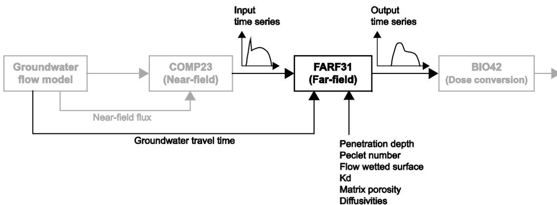
*Figure 1-1. Schematic illustration of the input and output of time series and parameters to and from FARF31.*
