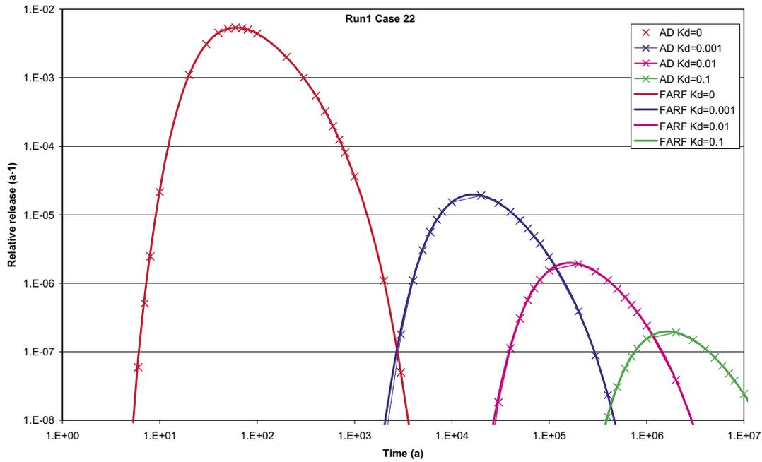
**Figure 4-2.** Comparison of an analytical solution of the advection dispersion equation with equilibrium sorption and results from FEARF31. Case B.
