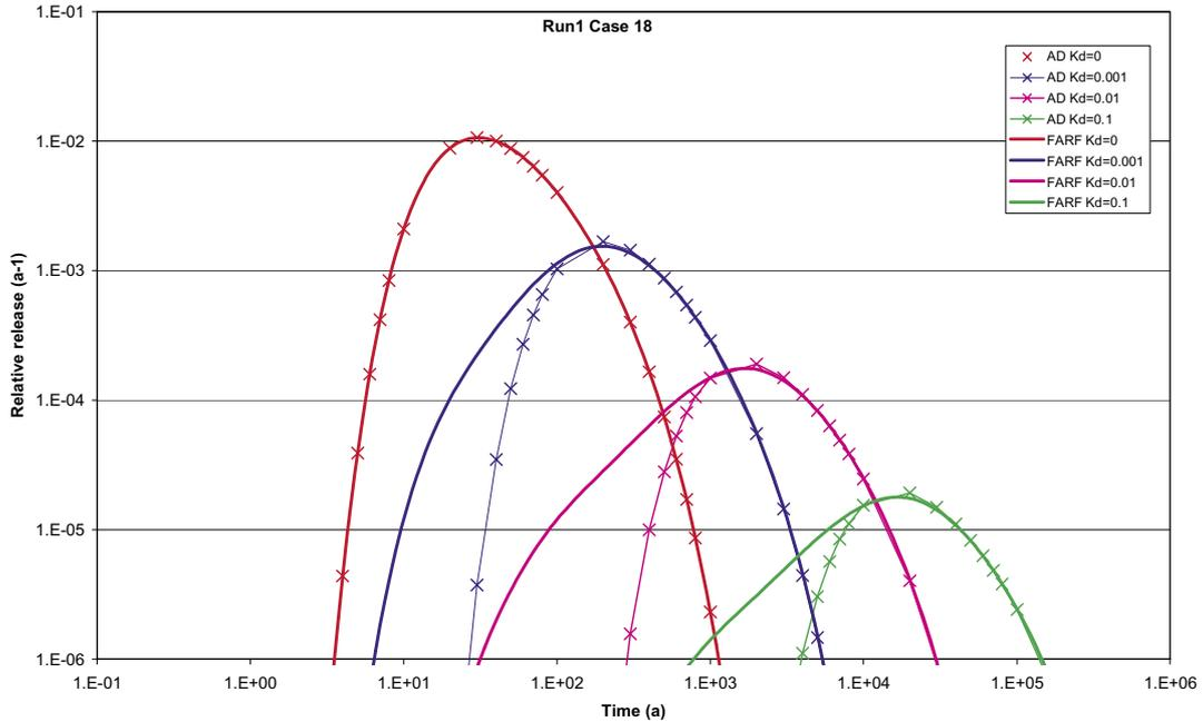
**Figure 4-1.** Comparison of an analytical solution of the advection dispersion equation with equilibrium sorption and results from FARF31. Case A.
