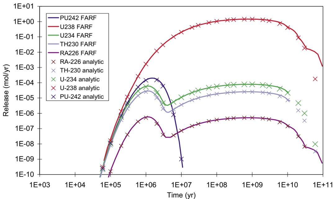
**Figure 4-6.** Comparison of release rates for chain 4N+2 calculated with an analytical method and FARF31.
