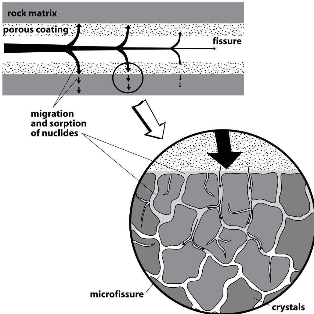
*Figure 2-1. Matrix diffusion and sorption in the microfissures in the rock matrix /Redrawn from Neretnieks, 1993/.*
