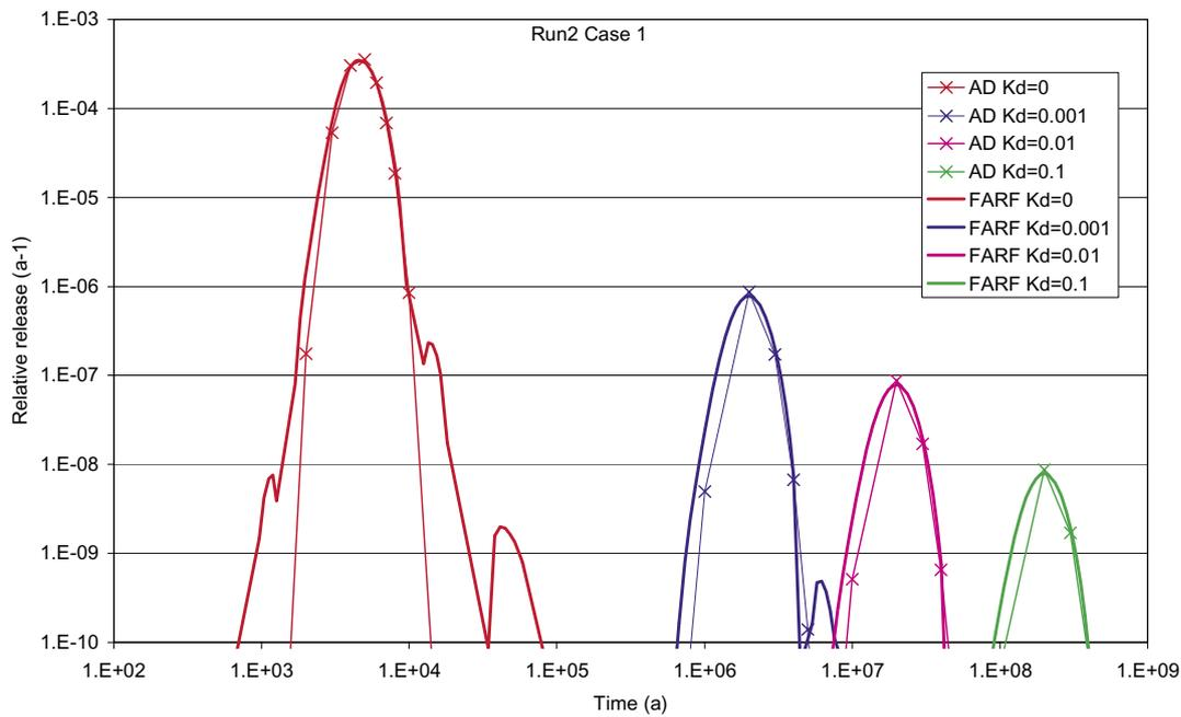
**Figure 4-3.** Comparison of an analytical solution of the advection dispersion equation with equilibrium sorption and results from FEARF31. Case C.
