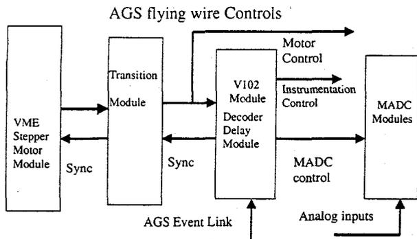
Figure 1: The AGS flying wire control sequence diagram.
