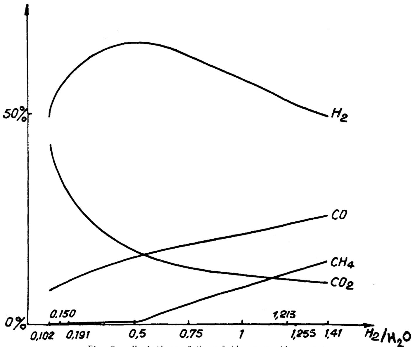
Fig. 2 — Variations of the relative proportion gases with quantity of water contained.
