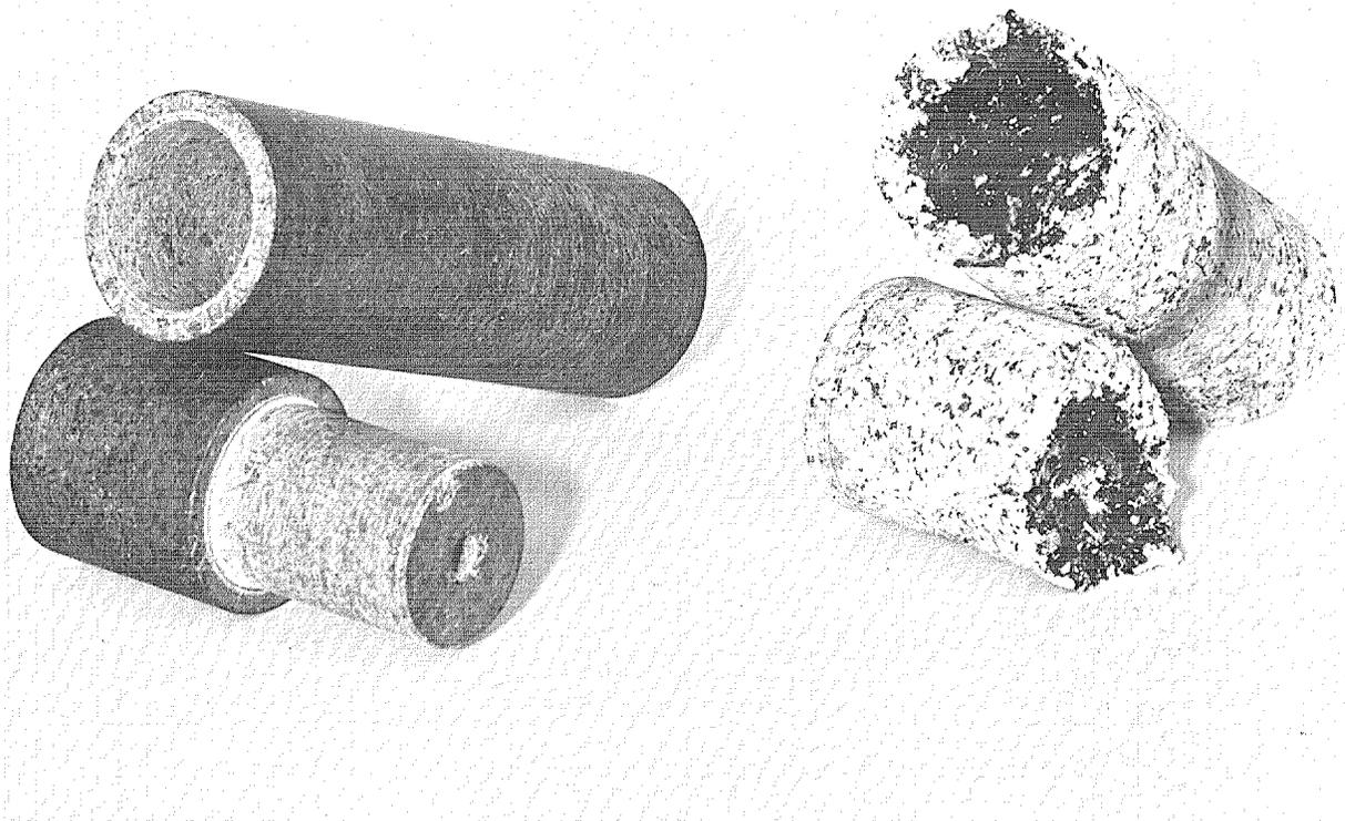
Fig. 5 Samples before and after plasmas heating.
